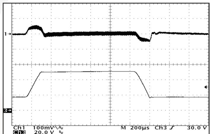
**Figure 12:** Output voltage response to step-change in input voltage (16V - 50V - 16V) in 150μs. Ch 1: Vout (100mV/div). Ch 3: Vin (20V/div).
