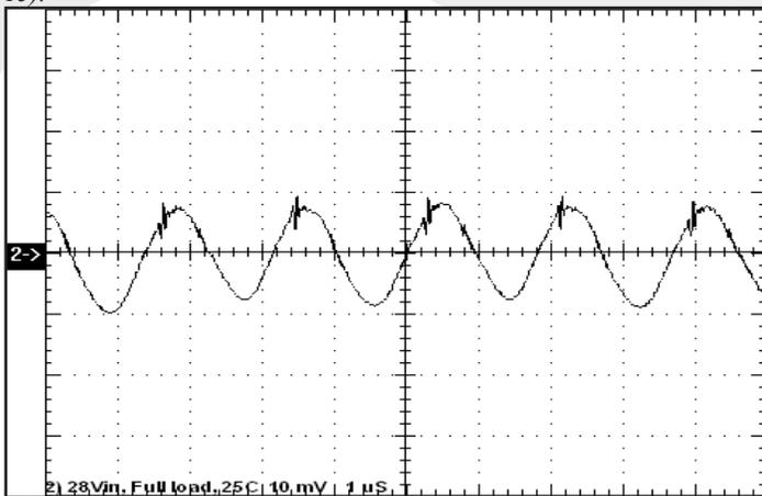
**Figure 15:** Output voltage ripple,  $V_{out}$ , at nominal input voltage and rated load current (10mV/div). Load capacitance: 1 $\mu$ F ceramic capacitor and 10 $\mu$ F tantalum capacitor. Bandwidth: 10MHz. See Figure 13.
