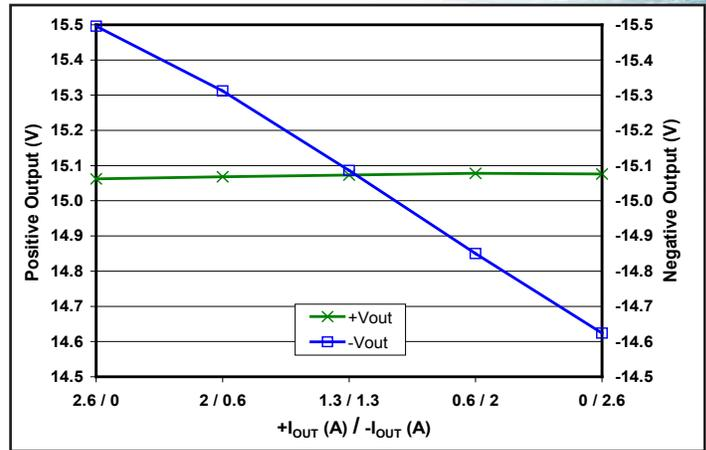
Figure 8: Load regulation vs. load current with power fixed at 80% load (40W) and load currents split as shown between the +15V and -15V outputs, at nominal input voltage and T<sub>case</sub> = 25°C.
