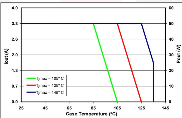
Figure 11: Output Current / Output Power derating curve as a function of T<sub>case</sub> and the Maximum desired power MOSFET junction temperature at V<sub>in</sub> = 28V (see Note 12).
