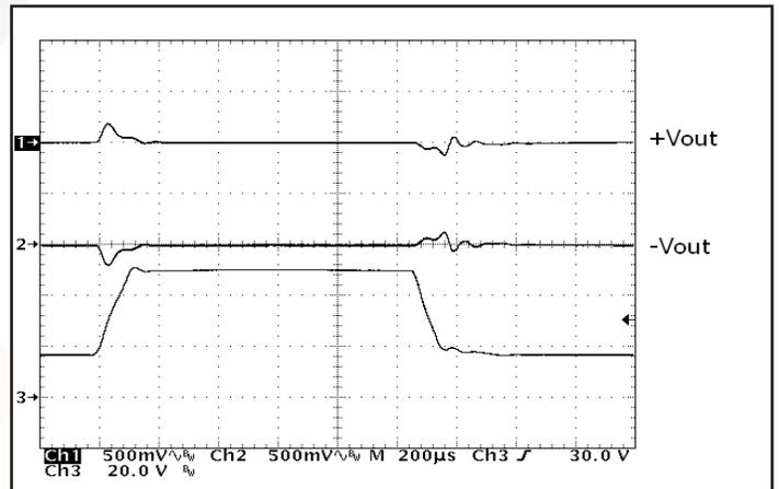
**Figure 18:** Output voltage response to step-change in input voltage (16V-50V-16V). Load cap: 1µF ceramic cap and 10µF, 100mΩ ESR tantalum cap. Ch 1: +Vout (500mV/div); Ch 2: -Vout (500mV/div); Ch 3: Vin (20V/div).
