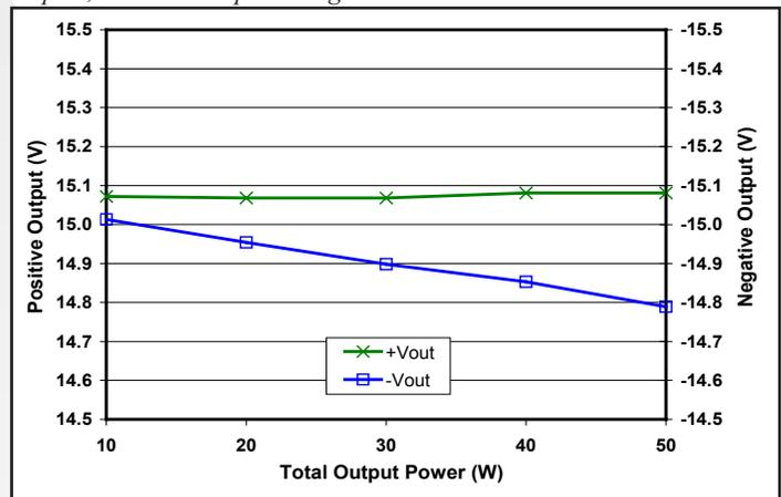
Figure 10: Load regulation vs. total output power where -I<sub>out</sub> equals three times +I<sub>out</sub> a nominal input voltage and T<sub>case</sub> = 25°C.
