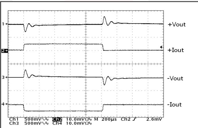
**Figure 17:** Output voltage response to step-change in total load current (0%-50%-0%) of total Iout (max) split 50%/50%. Load cap: 1µF ceramic cap and 10µF, 100mΩ ESR tantalum cap. Ch 1: +Vout (500mV/div); Ch 2: +Iout (2A/div); Ch 3: -Vout (500mV/div); Ch 4: -Iout (2A/div).
