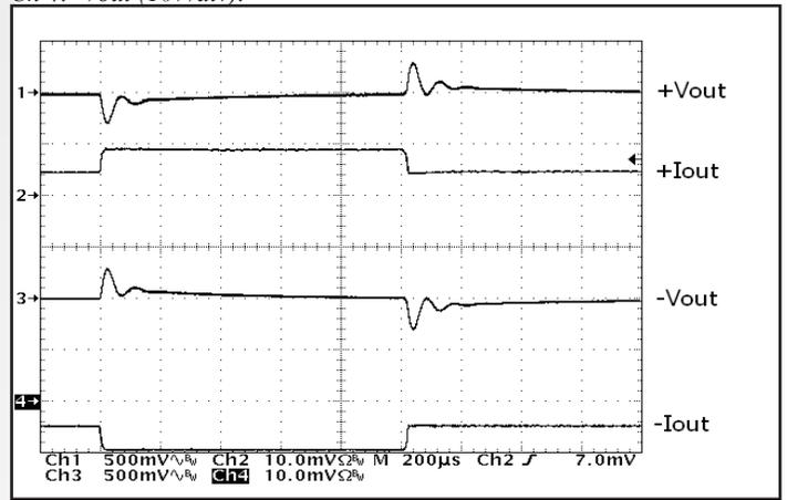
**Figure 16:** Output voltage response to step-change in total load current (50%-100%-50%) of total Iout (max) split 50%/50%. Load cap: 1µF ceramic cap and 10µF, 100mΩ ESR tantalum cap. Ch 1: +Vout (500mV/div); Ch 2: +Iout (2A/div); Ch 3: -Vout (500mV/div); Ch 4: -Iout (2A/div).
