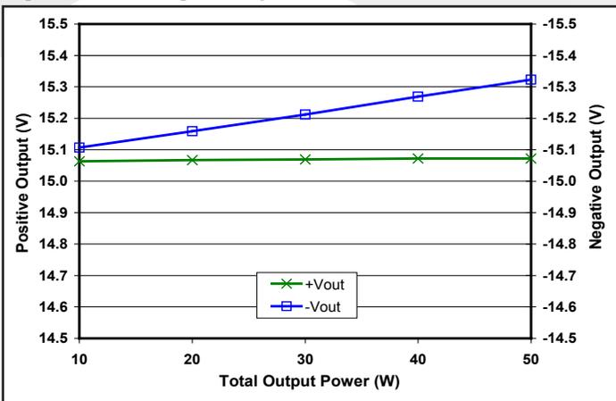
Figure 9: Load regulation vs. total output power where +I<sub>out</sub> equals three times -I<sub>out</sub> a nominal input voltage and T<sub>case</sub> = 25°C.
