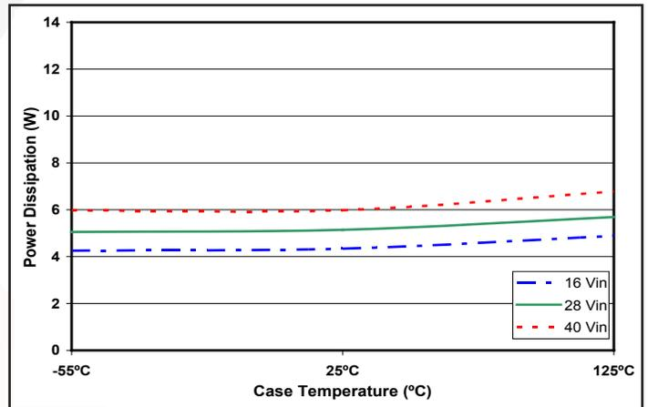
*Figure 5: Efficiency at 60% load (0.99A load on +15V and 0.99A load on -15V) versus case temperature for Vin = 16V, 28V and 40V.*
