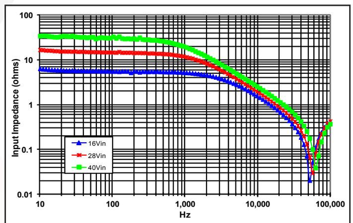
**Figure 30:** Magnitude of incremental input impedance ( $Z_{in} = v_{in}/i_{in}$ ) for minimum, nominal, and maximum input voltage at full rated power.
