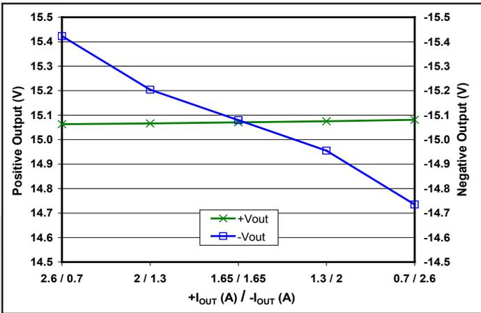
Figure 7: Load regulation vs. load current with power fixed at full load (50W) and load currents split as shown between the +15V and -15V outputs, at nominal input voltage and T<sub>case</sub> = 25°C.
