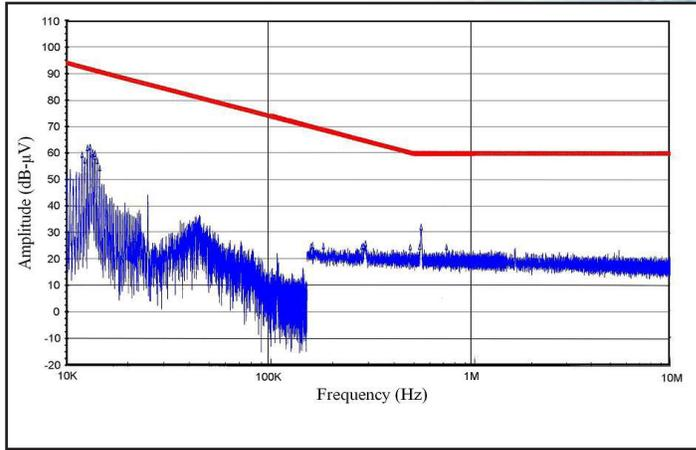
**Figure 32:** High frequency conducted emissions of MQHL-28-05S, 5Vout module at 50W output with MQHE-28-P filter, as measured with Method CE102. Limit line shown is the 'Basic Curve' for all applications with a 28V source.
