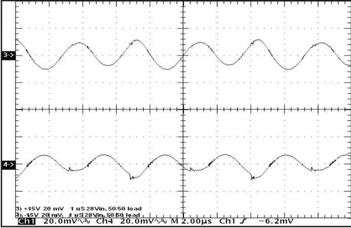
**Figure 21:** Output voltage ripple,  $+V_{out}$  (Ch 1) and  $-V_{out}$  (Ch 2), at nominal input voltage and full load current evenly split (20mV/div). Load capacitance:  $1\ \mu\text{F}$  ceramic cap and  $10\ \mu\text{F}$  tantalum cap.. Bandwidth; 10MHz. See Figure 19.
