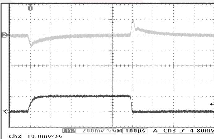
**Figure 11:** Output voltage response to step-change in load current 0%-50%-0% of Iout (max). Load cap: 1µF ceramic cap and 10µF, 100mΩ ESR tantalum cap. Ch 1: Vout (200mV/div). Ch 2: Iout (10A/div).
