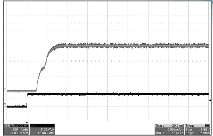
**Figure 8:** Turn-on transient at full resistive load and 5mF output capacitance initiated by ENAI. Input voltage pre-applied. Ch 1: Vout (500mV/div). Ch 3: ENAI (5V/div).
