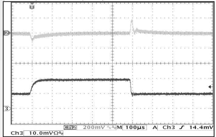
**Figure 10:** Output voltage response to step-change in load current 50%-100%-50% of Iout (max). Load cap: 1µF ceramic cap and 10µF, 100mΩ ESR tantalum cap. Ch 1: Vout (200mV/div). Ch 2: Iout (10A/div).
