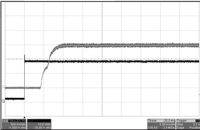
**Figure 9:** Turn-on transient at full resistive load and zero output capacitance initiated by Vin. ENAI previously high. Ch 1: Vout (500mV/div). Ch 3: Vin (10V/div).
