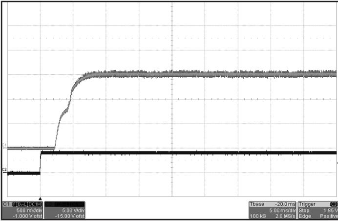
**Figure 7:** Turn-on transient at full resistive load and zero output capacitance initiated by ENAI. Input voltage pre-applied. Ch 1: Vout (500mV/div). Ch 3: ENAI (5V/div).
