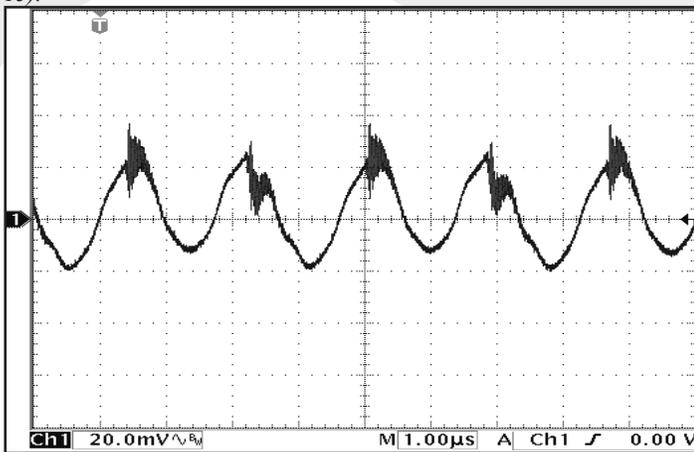
**Figure 15:** Output voltage ripple,  $V_{out}$ , at nominal input voltage and rated load current (20mV/div). Load capacitance: 1 $\mu F$  ceramic capacitor and 10 $\mu F$  tantalum capacitor. Bandwidth: 10MHz. See Figure 13.
