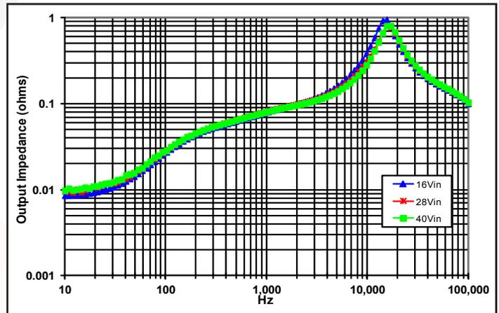
**Figure 24:** Magnitude of incremental output impedance of  $+15\text{V}$  output ( $+Z_{out} = +v_{out}/+i_{out}$ ) for minimum, nominal, and maximum input voltage at full rated power.
