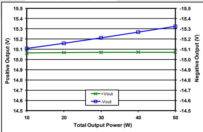
**Figure 9:** Load regulation vs. total output power where +Iout equals three times -Iout a nominal input voltage and  $T_{case} = 25^{\circ}C$ .
