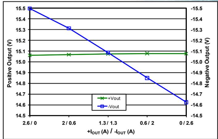
**Figure 8:** Load regulation vs. load current with power fixed at 80% load (40W) and load currents split as shown between the +15V and -15V outputs, at nominal input voltage and  $T_{case} = 25^{\circ}C$ .
