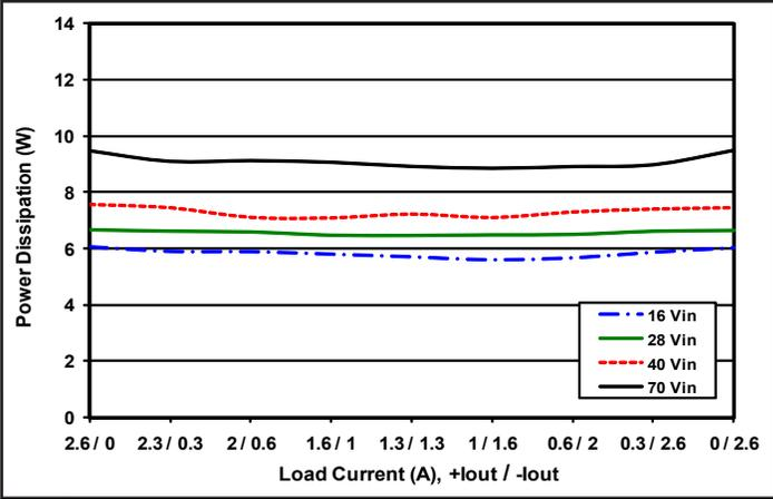
**Figure 4:** Power dissipation vs. output power, with total output current fixed at 80% load (40W) and loads split as shown between the +15V and -15V outputs at minimum, nominal, and maximum input voltage at Tcase=25°C.
