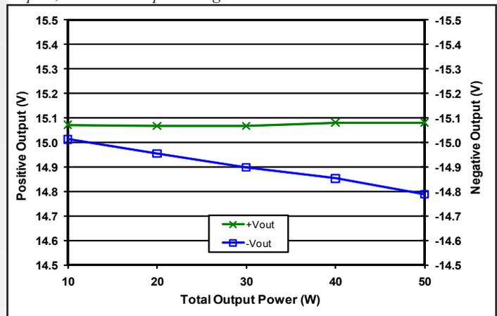
**Figure 10:** Load regulation vs. total output power where -Iout equals three times +Iout a nominal input voltage and  $T_{case} = 25^{\circ}C$ .
