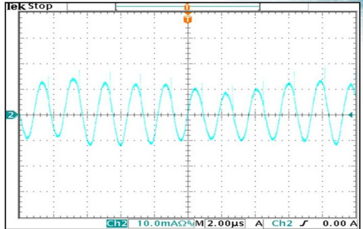
**Figure 14:** Input terminal current ripple,  $i_c$ , at full rated output current and nominal input voltage with SynQor MQ filter module (10mA/div). Bandwidth: 20MHz. Timebase: (2 $\mu$ s/div). See Figure 13.
