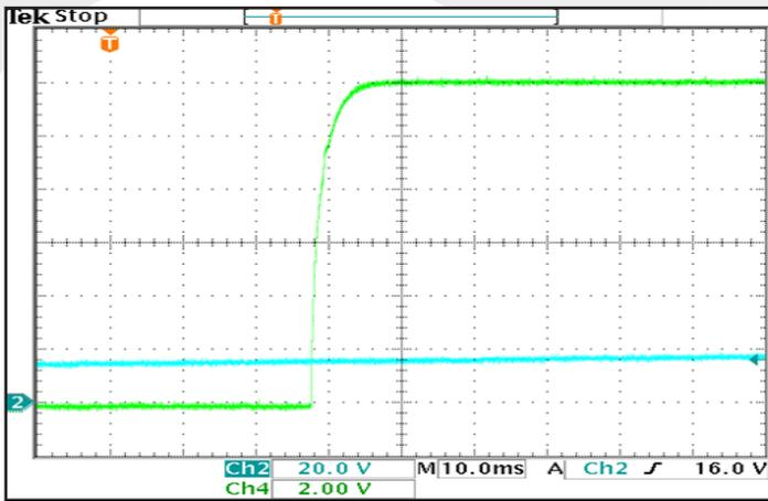
**Figure 9:** Turn-on transient at full resistive load and zero output capacitance initiated by Vin. ENA1 previously high. Ch 2: Vin (20V/div). Ch 4: Vout (2V/div). Timebase: (10ms/div).
