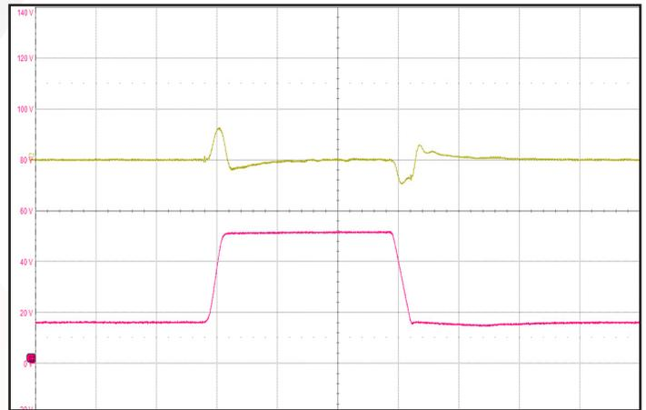
**Figure 12:** Output voltage response to step-change in input voltage (16V - 50V - 16V) in 150µs. Ch 1: Vout (200mV/div). Ch 2: Vin (20V/div). Bandwidth: 20MHz. Timebase: (500us/div).
