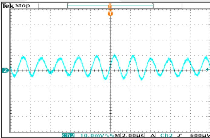
**Figure 15:** Output voltage ripple,  $V_{out}$ , at nominal input voltage and rated load current (10mV/div). Load capacitance: 1 $\mu$ F ceramic capacitor and 10 $\mu$ F tantalum capacitor. Bandwidth: 20MHz. Timebase: (2 $\mu$ s/div). See Figure 13.
