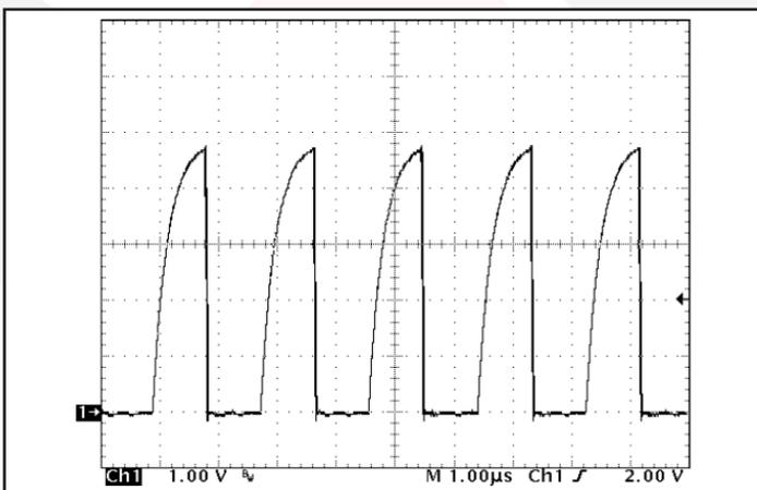
**Figure 17:** SYNC OUT vs. time, driving SYNC IN of a second SynQor MQHL converter. Ch1: SYNC OUT: (1V/div). Timebase: (1 $\mu$ s/div).
