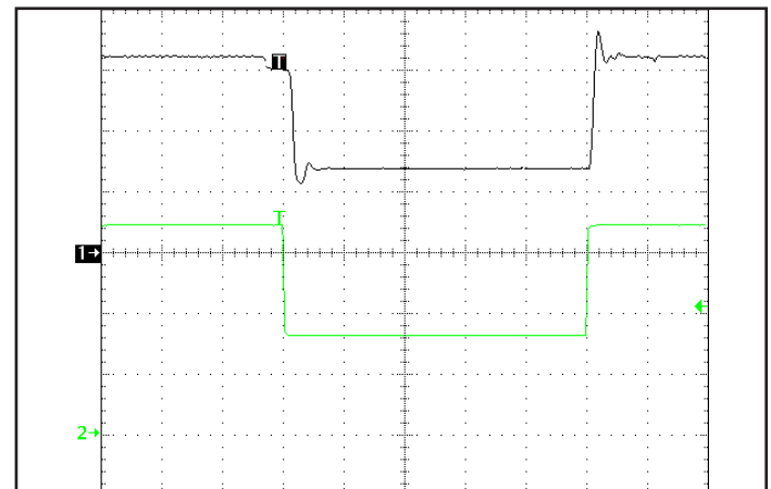
Figure 12: Output Current vs. I_{set} pin voltage dynamics; 28Vin 5Vout (5ms/div). Top Trace: Output Current (5A/div). Bottom Trace: I_{set} pin voltage (500mV/div)
