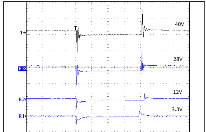
Figure 14: Output voltage response for 28V input; 3.3V, 12V, 28V, 40V output to step change in load current (50%-75%-50% of I out max; di/dt=0.1A/μs). Load cap: 100μF electrolytic cap, V out (500mV/div); (5mS/div)
