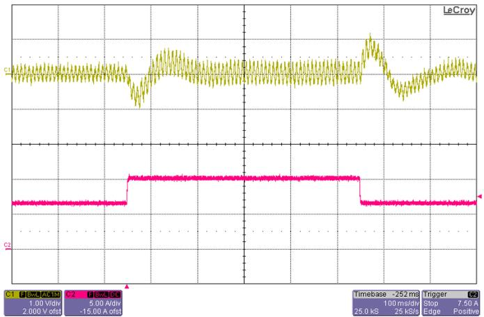
**Figure 8:** Output voltage response to step-change in load current with 200µF hold-up capacitor (50%-75%-50% of Iout(max), 115Vrms, 60Hz) Top: Vout (1V/div), Bottom: Iout (5A/div), Timebase: (100ms/div).
