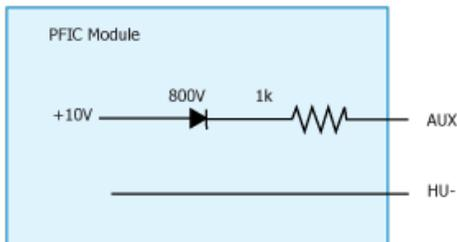
The purpose of the AUX power supply is to provide a low level of power to primary control circuitry, referenced to HU-.
