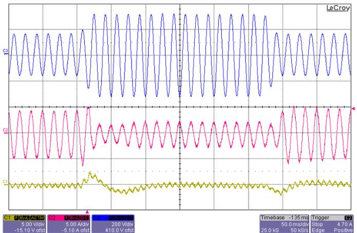
**Figure 10:** Input voltage transient response with 200µF hold-up capacitor at full load current (115Vrms-230Vrms-115Vrms, 60Hz), Top: Vin (200V/div), Mid: Iin (5A/div), Bottom: Vout (5V/div), Timebase: (50ms/div).
