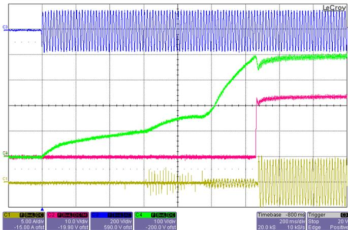
**Figure 9:** Typical startup waveform with 200µF hold-up capacitor (115Vrms, 60Hz) Ch1: Iin (5A/div), Ch2: Vout (10V/div), Ch3: Vin (200V/div), Ch4: Hold-up capacitor voltage (100V/div), Timebase: (200ms/div).
