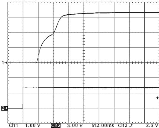
Figure 9: Turn-on transient at full load (resistive load) (2 ms/div). Input voltage pre-applied. Ch 1: V<sub>out</sub> (1V/div). Ch 2: ON/OFF input (5V/div)
