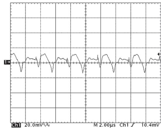
Figure 16: Output voltage ripple at nominal input voltage and rated load current ( $20 \text{ mV}/\text{div}$ ). Load capacitance:  $1 \mu\text{F}$  ceramic capacitor and  $10 \mu\text{F}$  tantalum capacitor. Bandwidth:  $20 \text{ MHz}$ . See Figure 13.
