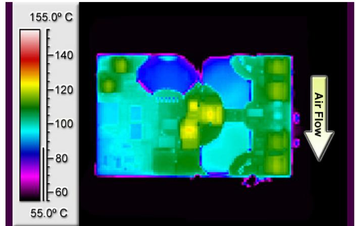
Figure 8: Thermal plot of converter at 19 amp load current with 55°C air flowing at the rate of 200 LFM. Air is flowing across the converter from pin 1 to pin 3 (nominal input voltage).
