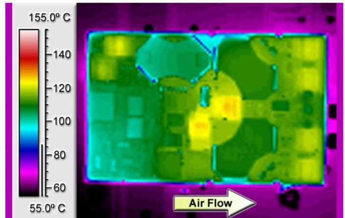
Figure 6: Thermal plot of converter at 20 amp load current with 55°C air flowing at the rate of 200 LFM. Air is flowing across the converter from input to output (nominal input voltage).
