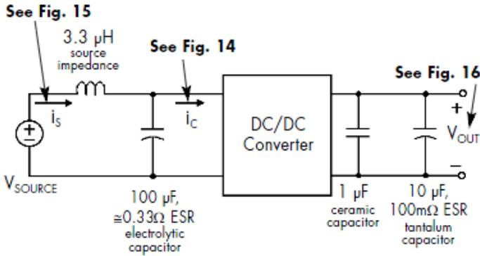
Figure 13: Test set-up diagram showing measurement points for Input Terminal Ripple Current (Figure 14), Input Reflected Ripple Current (Figure 15) and Output Voltage Ripple (Figure 16).
