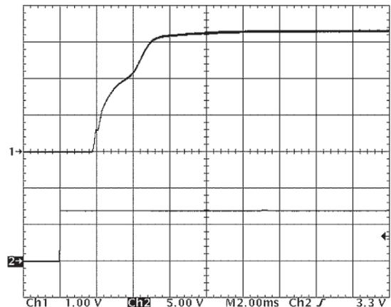
Figure 10: Turn-on transient at zero load (2 ms/div). Ch 1: V<sub>out</sub> (1V/div) Ch 2: ON/OFF input (5V/div)
