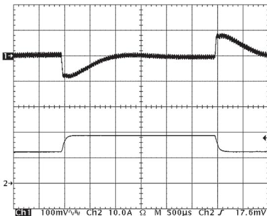
Figure 11: Output voltage response to step-change in load current (50%-75%-50% of I<sub>out</sub>(max); dI/dt = 0.1A/μs). Load cap: 10μF, 100 mΩ ESR tantalum capacitor and 1μF ceramic capacitor. Ch 1: V<sub>out</sub> (100mV/div), Ch 2: I<sub>out</sub> (10A/div).
