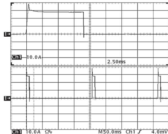
Figure 18: Load current ( $10 \text{ A}/\text{div}$ ) as a function of time when the converter attempts to turn on into a  $10 \text{ m}\Omega$  short circuit. Top trace ( $2.5 \text{ ms}/\text{div}$ ) is an expansion of the on-time portion of the bottom trace.
