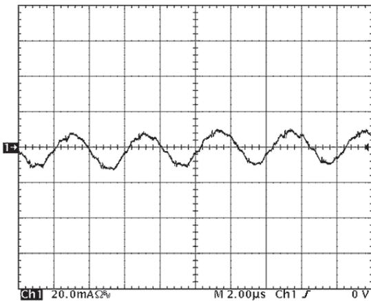
Figure 15: Input reflected ripple current,  $i_s$ , through a  $3.3 \mu\text{H}$  source inductor at nominal input voltage and rated load current ( $20 \text{ mA}/\text{div}$ ). See Figure 13.
