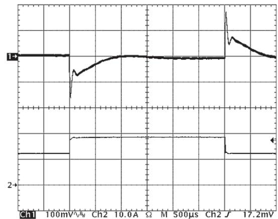
Figure 12: Output voltage response to step-change in load current (50%-75%-50% of I<sub>out</sub>(max); dI/dt = 5A/μs). Load cap: 470μF, 30 mΩ ESR tantalum capacitor and 1μF ceramic cap. Ch 1: V<sub>out</sub> (100mV/div), Ch 2: I<sub>out</sub> (10A/div).
