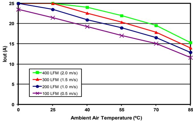
Figure 7: Maximum output power-derating curves vs. ambient air temperature for airflow rates of 0 LFM through 400 LFM with air flowing from pin 1 to pin 3 (nominal input voltage).
