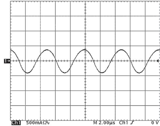
Figure 14: Input Terminal Ripple Current,  $i_s$ , at full rated output current and nominal input voltage with  $3.3 \mu\text{H}$  source impedance and  $100 \mu\text{F}$  electrolytic capacitor ( $500 \text{ mA}/\text{div}$ ). See Figure 13.
