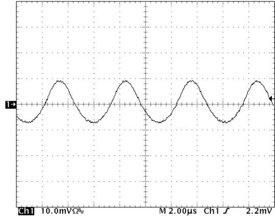
Figure 14: Input Terminal Ripple Current,  $i_c$ , at full rated output current and nominal input voltage with  $10\ \mu\text{H}$  source impedance and  $47\ \mu\text{F}$  electrolytic capacitor (500 mA/div). See Figure 13
