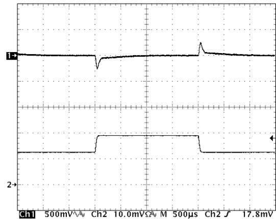
Figure 12: Output voltage response to step-change in load current (50%-75%-50% of I<sub>out</sub>(max); dI/dt = 0.4A/μs). Load cap: 470μF, 30 mΩ ESR tantalum capacitor and 1μF ceramic cap. Ch 1: V<sub>out</sub> (500mV/div), Ch 2: I<sub>out</sub> (10A/div).
