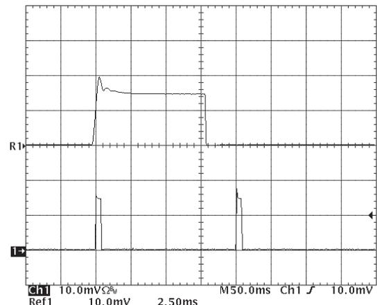
Figure 18: Load current (20A/div) as a function of time when the converter attempts to turn on into a  $1\ \text{m}\Omega$  short circuit. Top trace (2.5ms/div) is an expansion of the on-time portion of the bottom trace.
