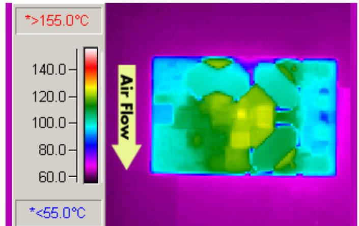
Figure 6: Thermal plot of converter at 23.5 amp load current with 55°C air flowing at the rate of 200 LFM. Air is flowing across the converter from pin 1 to pin 3 (nominal input voltage).
