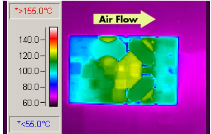
Figure 8: Thermal plot of converter at 23 amp load current with 55°C air flowing at the rate of 200 LFM. Air is flowing across the converter from input to output (nominal input voltage).
