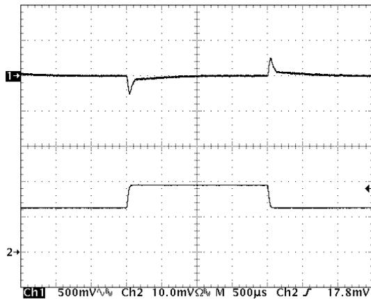
Figure 11: Output voltage response to step-change in load current (50%-75%-50% of I<sub>out</sub>(max); dI/dt = 0.16A/μs). Load cap: 10μF, 100 mΩ ESR tantalum capacitor and 1μF ceramic capacitor. Ch 1: V<sub>out</sub> (500mV/div), Ch 2: I<sub>out</sub> (10A/div).
