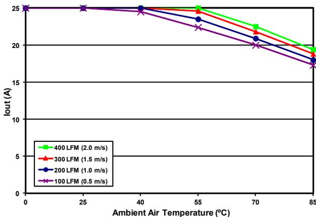
Figure 5: Maximum output power derating curves vs. ambient air temperature for airflow rates of 100 LFM through 400 LFM with air flowing from pin 1 to pin 3 (nominal input voltage).
