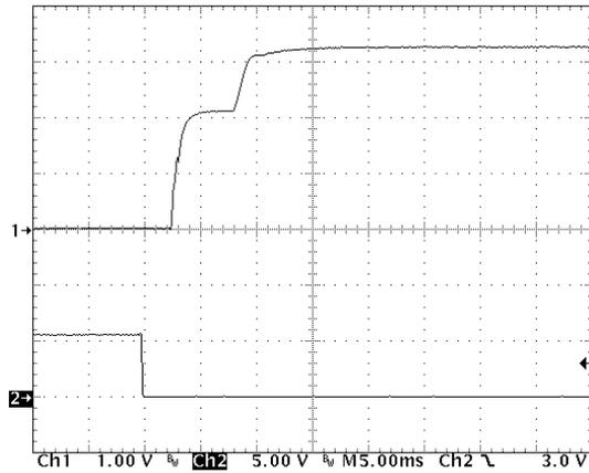
Figure 9: Turn-on transient at full load (resistive load) (5 ms/div). Input voltage pre-applied. Ch 1: V<sub>out</sub> (1V/div). Ch 2: ON/OFF input (5V/div)
