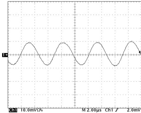
Figure 15: Input reflected ripple current,  $i_s$ , through a  $10\ \mu\text{H}$  source inductor at nominal input voltage and rated load current (10 mA/div). See Figure 13.
