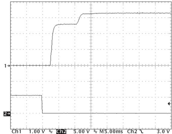
Figure 10: Turn-on transient at zero load (5 ms/div). Ch 1: V<sub>out</sub> (1V/div) Ch 2: ON/OFF input (5V/div)
