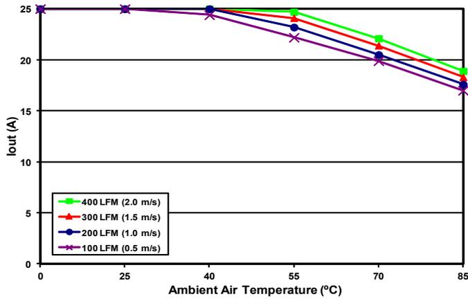
Figure 7: Maximum output power-derating curves vs. ambient air temperature for airflow rates of 100 LFM through 400 LFM with air flowing from input to output (nominal input voltage).
