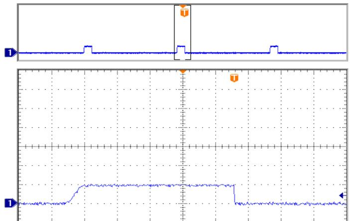
**Figure 18: Output Short Load Current** (50A/div) as a function of time when the converter attempts to turn on into a  $1 m\Omega$  short circuit. Top trace (200ms/div) is an expansion of the on-time portion of the bottom trace.
