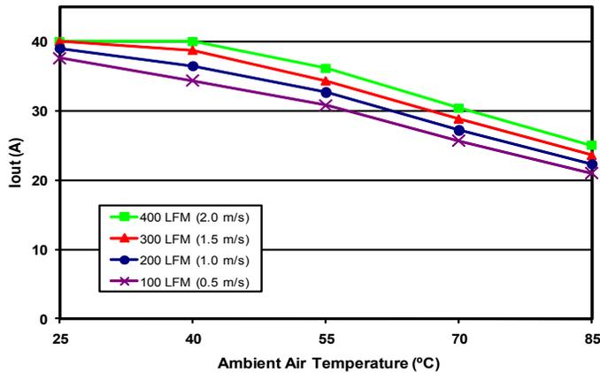
**Figure 7: Thermal Derating** (max output current vs. ambient air temperature) for airflow rates of 100 LFM through 400 LFM with air flowing lengthwise from output to input (nominal input voltage).
