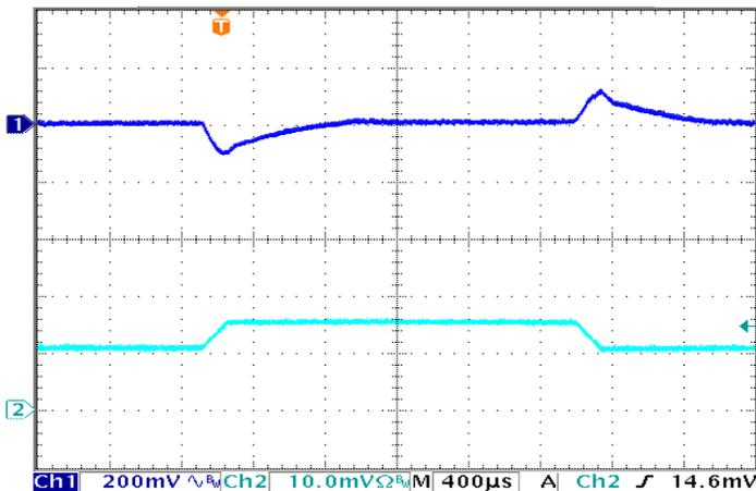
**Figure 11: Output Voltage Response** to Step-Change in Load Current (50%-75%-50% of Iout(max); dI/dt = 0.1A/us). Load cap: 100µF electrolytic output capacitance. Top trace: Vout (200mV/div). Bottom trace: Iout (20A/div).
