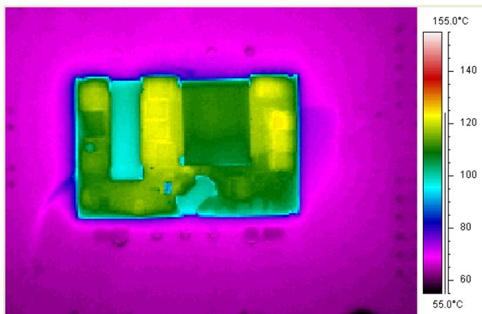
Figure 6: Thermal Image of converter at 34.0 amp load current (170W) with 55°C air flowing at the rate of 200 LFM. Air is flowing from pin 3 to pin 1 (nominal input voltage).
