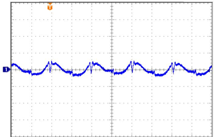
**Figure 16: Output Ripple** at nominal input voltage and rated load current (50 mV/div). Load capacitance: one  $1.0\mu F$  ceramic capacitor and one  $100\mu F$  electrolytic capacitor. Bandwidth: 20 MHz. (See Figure 13).
