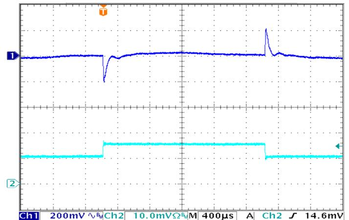
**Figure 12: Output Voltage Response** to Step-Change in Load Current (50%-75%-50% of Iout(max); dI/dt = 5A/us). Load cap: 330µF electrolytic output capacitance. Top trace: Vout (200mV/div). Bottom trace: Iout (20A/div).
