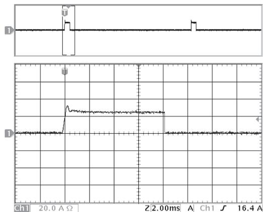
Figure 18: Load current (20A/div) as a function of time when the converter attempts to turn on into a 10 m $\Omega$  short circuit. Top trace (2.5ms/div) is an expansion of the on-time portion of the bottom trace.
