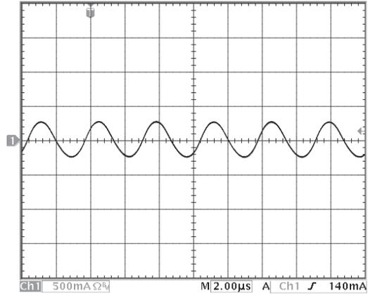
Figure 14: Input Terminal Ripple Current,  $i_s$ , at full rated output current and nominal input voltage with 3.3 $\mu\text{H}$  source impedance and 100 $\mu\text{F}$  electrolytic capacitor (500 mA/div). See Figure 13.
