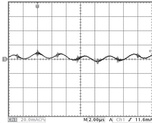
Figure 15: Input reflected ripple current,  $i_s$ , through a 3.3  $\mu\text{H}$  source inductor at nominal input voltage and rated load current (20 mA/div). See Figure 13.
