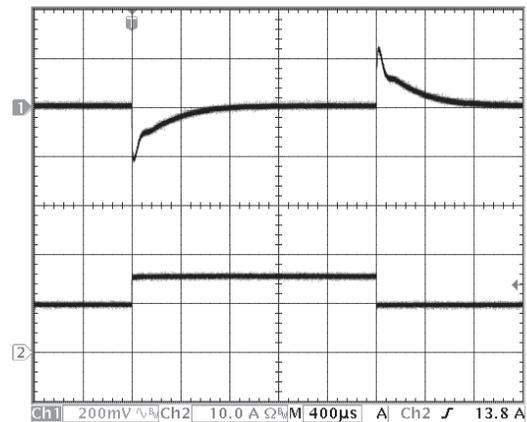
Figure 12: Output voltage response to step-change in load current (50%-75%-50% of  $I_{out(max)}$ ;  $dI/dt = 5\text{A}/\mu\text{s}$ ). Load cap: 470 $\mu\text{F}$ , 30 m $\Omega$  ESR tantalum capacitor and 1 $\mu\text{F}$  ceramic cap. Ch 1:  $V_{out}$  (200mV/div), Ch 2:  $I_{out}$  (10A/div)
