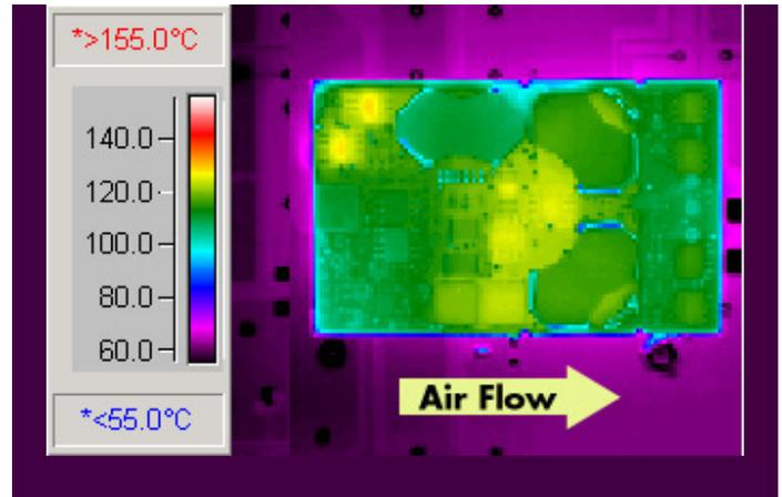
Figure 8: Thermal plot of converter at 14 amp load current (70W) with 55°C air flowing at the rate of 200 LFM. Air is flowing across the converter from input to output (nominal input voltage).
