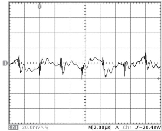
Figure 16: Output voltage ripple at nominal input voltage and rated load current (20 mV/div). Load capacitance: 1 $\mu\text{F}$  ceramic capacitor and 10 $\mu\text{F}$  tantalum capacitor. Bandwidth: 20 MHz. See Figure 13.
