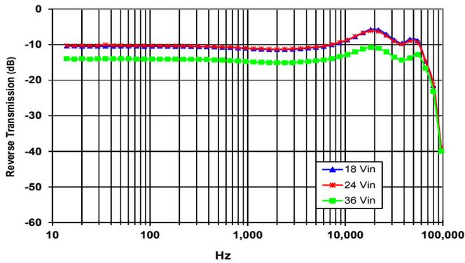
Figure 21: Magnitude of incremental reverse transmission ( $RT = i_{in}/i_{out}$ ) for minimum, nominal, and maximum input voltage at full rated power.
