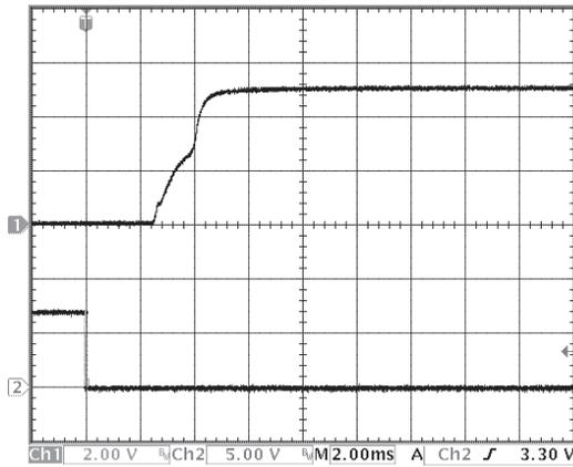
Figure 9: Turn-on transient at full load (resistive load) (2 ms/div). Input voltage pre-applied. Ch 1:  $V_{out}$  (2V/div). Ch 2: ON/OFF input (5V/div)
