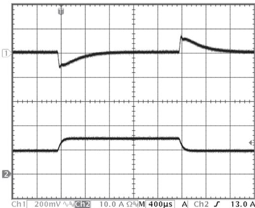
Figure 11: Output voltage response to step-change in load current (50%-75%-50% of  $I_{out(max)}$ ;  $dI/dt = 0.1\text{A}/\mu\text{s}$ ). Load cap: 10 $\mu\text{F}$ , 100 m $\Omega$  ESR tantalum capacitor and 1 $\mu\text{F}$  ceramic capacitor. Ch 1:  $V_{out}$  (200mV/div), Ch 2:  $I_{out}$  (10A/div)
