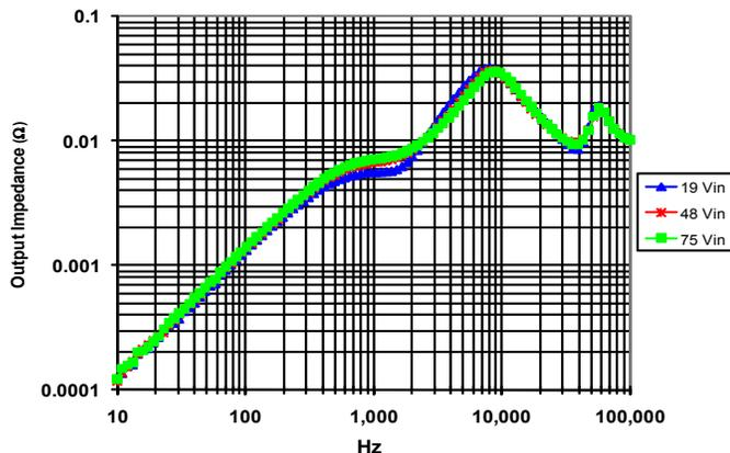
Figure 23: Magnitude of incremental output impedance ( $Z_{out} = V_{out}$ ) for minimum, nominal, and maximum input voltage at full rated power.
