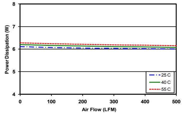
Figure 4: Power dissipation at nominal output voltage and 60% rated power vs. airflow rate for ambient air temperatures of 25°C, 40°C, and 55°C (48V input).
