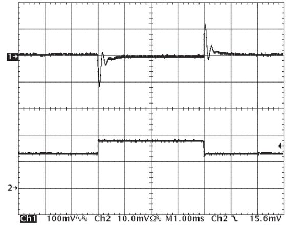
Figure 16: Output voltage response to step-change in load current (50%-75%-50% of  $I_{out(max)}$ ;  $dI/dt = 5A/\mu s$ ). Load cap  $470\mu F$ ,  $30\text{ m}\Omega$  ESR tantalum cap and  $1\mu F$  ceramic cap. Ch 1: Vout (100mV/div), Ch 2: Iout (10A/div).
