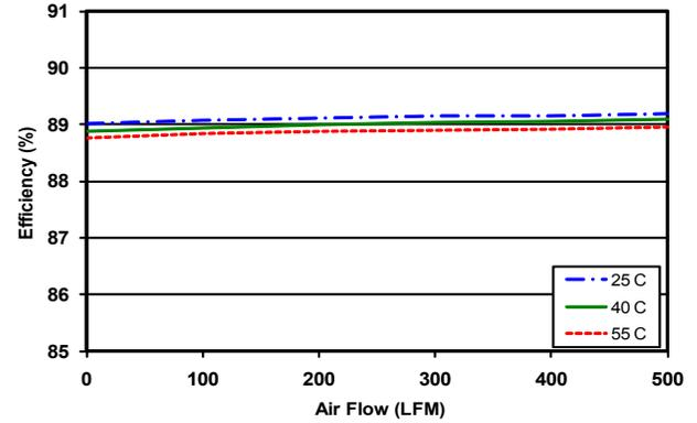
Figure 2: Efficiency at nominal output voltage and 60% rated power vs. airflow rate for ambient air temperatures of 25°C, 40°C and 55°C (48V input).
