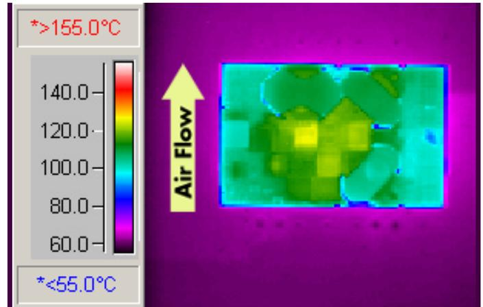
Figure 8: Thermal plot of converter at 25 amp load current with 55°C air flowing at the rate of 200 LFM. Air is flowing across the converter from pin 3 to pin 1 (48V input).
