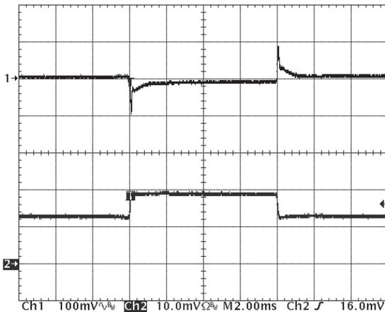
Figure 15: Output voltage response to step-change in load current (50%-75%-50% of  $I_{out(max)}$ ;  $dI/dt = 0.1A/\mu s$ ). Load cap:  $10\mu F$ ,  $100\text{ m}\Omega$  ESR tantalum cap and  $1\mu F$  ceramic cap. Ch 1: Vout (100mV/div), Ch 2: Iout (10A/div).
