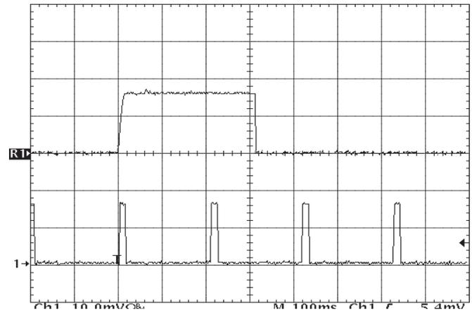
Figure 22: Load Current (20A/div) as a function of time when the converter attempts to turn on into a  $10 \text{ m}\Omega$  short circuit. Top trace (5ms/div) is an expansion of the on-time portion of the bottom trace.
