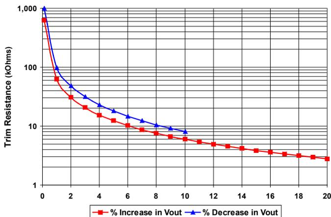
Figure C: Trim Graph for 2.0V<sub>out</sub> module
