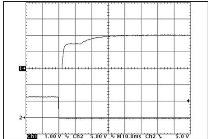
Figure 10: Turn-on transient at zero load (10 ms/div).
