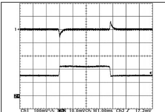
Figure 11: Output voltage response to step-change in load current (50%-75%-50% of I<sub>out</sub>(max); dI/dt = 0.1A/μs). Load cap: 15μF, 450 mΩ ESR tantalum capacitor and 1μF ceramic capacitor. Top trace: V<sub>out</sub> (100mV/div), Bottom trace: I<sub>out</sub> (10A/div).
