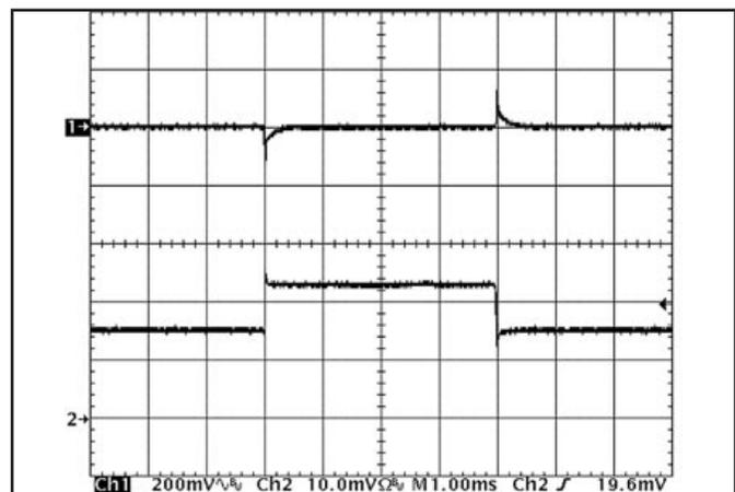
Figure 12: Output voltage response to step-change in load current (50%-75%-50% of I<sub>out</sub>(max); dI/dt = 5A/μs). Load cap: 480μF, 15 mΩ ESR tantalum capacitor and 1μF ceramic capacitor. Top trace: V<sub>out</sub> (200mV/div), Bottom trace: I<sub>out</sub> (10A/div).
