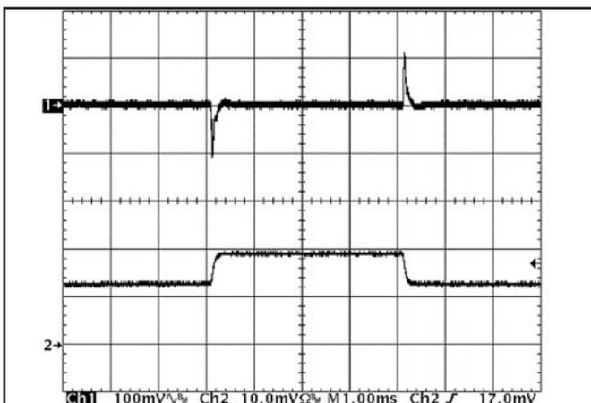
Figure 11: Output voltage response to step-change in load current (50%-75%-50% of Iout(max); dI/dt = 0.1A/μs). Load cap: 15μF, 450 mΩ ESR tantalum cap and 1μF ceramic cap. Top trace: Vout (100mV/div), Bottom trace: Iout (15A/div).
