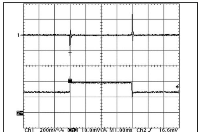
Figure 12: Output voltage response to step-change in load current (50%-75%-50% of Iout(max); dI/dt = 5A/μs). Load cap: 480μF, 15 mΩ ESR tantalum cap and 1μF ceramic cap. Top trace: Vout (200mV/div), Bottom trace: Iout (15A/div).
