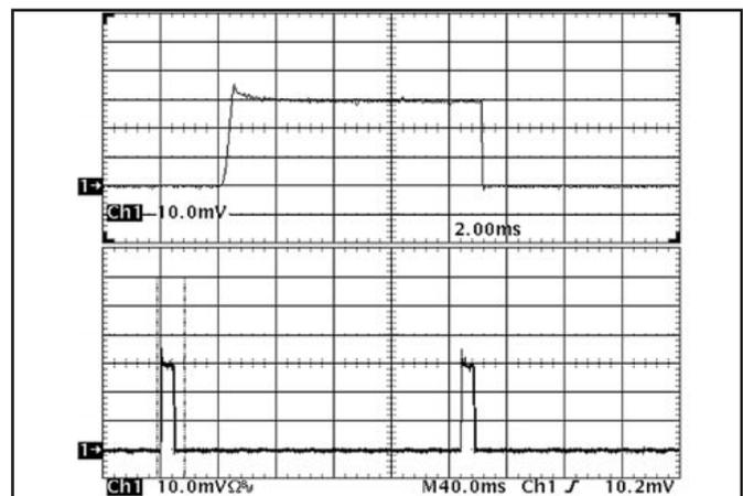
**Figure 18:** Load current ( $15\ \text{A}/\text{div}$ ) as a function of time when the converter attempts to turn on into a  $1\ \text{m}\Omega$  short circuit. Top trace ( $2\ \text{ms}/\text{div}$ ) is an expansion of the on-time portion of the bottom trace.
