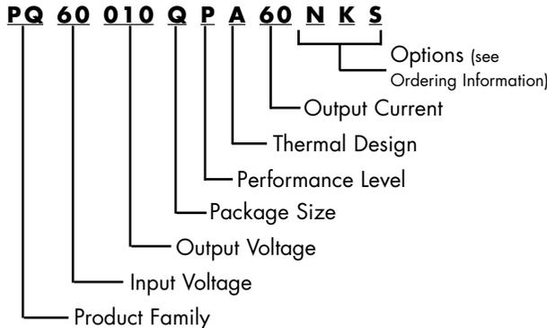
The first 12 characters comprise the base part number and the last 3 characters indicate available options. Although there are no default values for enable logic and pin length, the most common options are negative logic and 0.145" pins. These part numbers are more likely to be readily available in stock for evaluation and prototype quantities. A "-G" suffix indicates 6/6 RoHS compliance.
