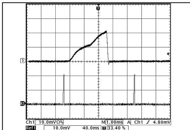
**Figure 18:** Load current (50A/div) as a function of time when the converter attempts to turn on into a  $1\ \text{m}\Omega$  short circuit. Top trace (1.0ms/div) is an expansion of the on-time portion of the bottom trace.
