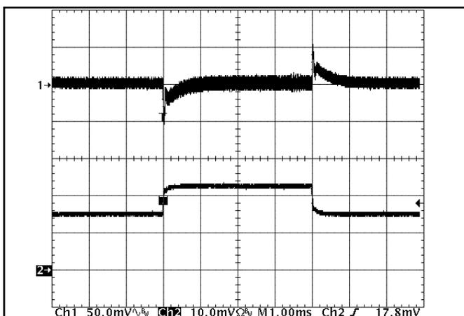
**Figure 11:** Output voltage response to step-change in load current (50%-75%-50% of  $I_{out(max)}$ ;  $dI/dt = 0.1\text{A}/\mu\text{s}$ ). Load cap: 10 $\mu\text{F}$ , 100 m $\Omega$  ESR tantalum cap and 1 $\mu\text{F}$  ceramic cap. Ch 1:  $V_{out}$  (50mV/div), Ch 2:  $I_{out}$  (20A/div).
