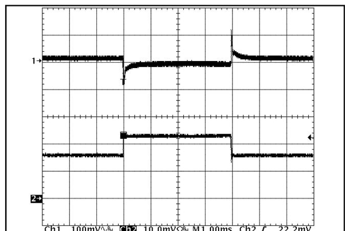
**Figure 12:** Output voltage response to step-change in load current (50%-75%-50% of  $I_{out(max)}$ ;  $dI/dt = 5\text{A}/\mu\text{s}$ ). Load cap: 470 $\mu\text{F}$ , 30 m $\Omega$  ESR tantalum cap and 1 $\mu\text{F}$  ceramic cap. Ch 1:  $V_{out}$  (100mV/div), Ch 2:  $I_{out}$  (20A/div).
