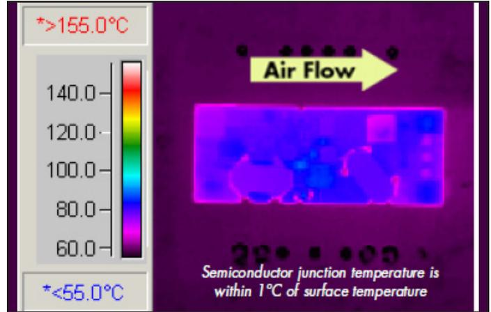
Figure 8: Thermal plot of converter at 25 amp load current with 55°C air flowing at the rate of 200 LFM. Air is flowing across the converter from input to output (nominal input voltage).
