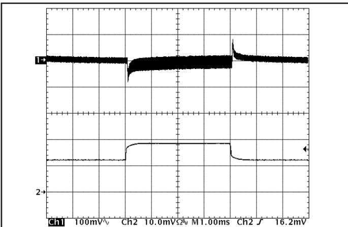
Figure 11: Output voltage response to step-change in load current (50%-75%-50% of  $I_{out(max)}$ ;  $dI/dt = 0.1\text{A}/\mu\text{s}$ ). Load cap: 10  $\mu\text{F}$ , 100 m $\Omega$  ESR tantalum cap and 1 $\mu\text{F}$  ceramic cap. Ch 1:  $V_{out}$  (100 mV/div). Ch 2:  $I_{out}$  (10 A/div).
