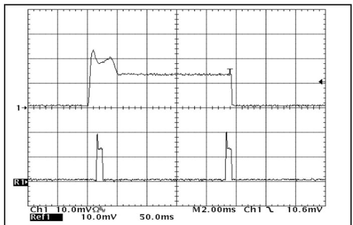
Figure 18: Load current (20 A/div) as a function of time when the converter attempts to turn on into a  $10\text{m}\Omega$  short circuit. Top trace (2.0 ms/div) is an expansion of the on-time portion of the bottom trace.
