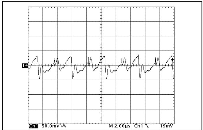
Figure 16: Output voltage ripple at nominal input voltage and rated load current (50 mV/div). Load capacitance:  $1\mu\text{F}$  ceramic capacitor and  $10\mu\text{F}$  tantalum capacitor. Bandwidth: 20 MHz. See Figure 13.
