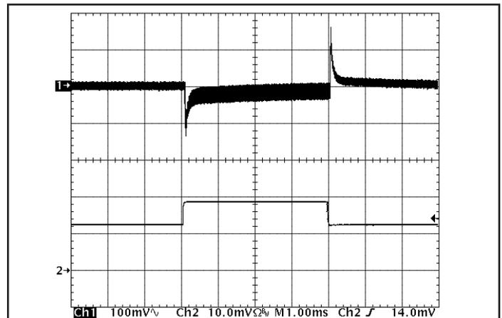
Figure 12: Output voltage response to step-change in load current (50%-75%-50% of  $I_{out(max)}$ ;  $dI/dt = 5\text{A}/\mu\text{s}$ ). Load cap: 470  $\mu\text{F}$ , 30 m $\Omega$  ESR tantalum cap and 1  $\mu\text{F}$  ceramic cap. Ch 1:  $V_{out}$  (100 mV/div). Ch 2:  $I_{out}$  (10 A/div).
