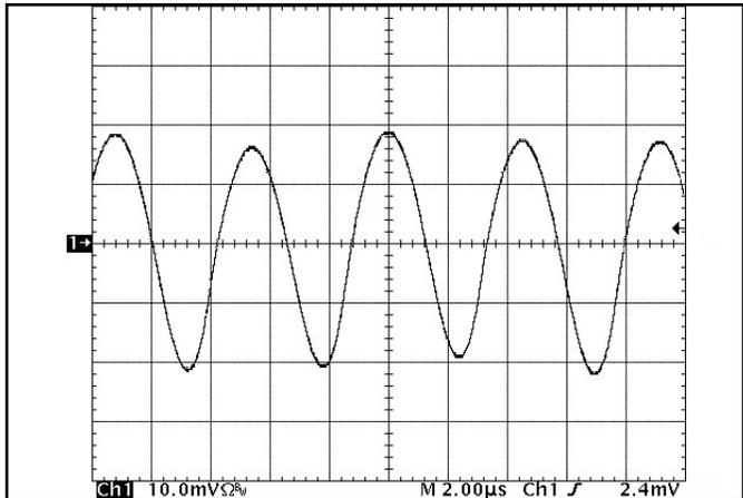
**Figure 14:** Input Terminal Ripple Current,  $i_c$ , at full rated output current and nominal input voltage with  $10\ \mu\text{H}$  source impedance and  $47\ \mu\text{F}$  electrolytic capacitor ( $100\ \text{mA}/\text{div}$ ). See Figure 13.
