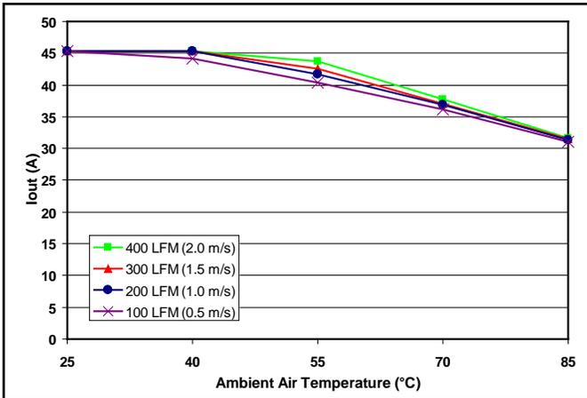
**Figure 7:** Maximum output power derating curves vs. ambient air temperature for airflow rates of 100 LFM through 400 LFM with air flowing across the converter from pin input to output (nominal input voltage).
