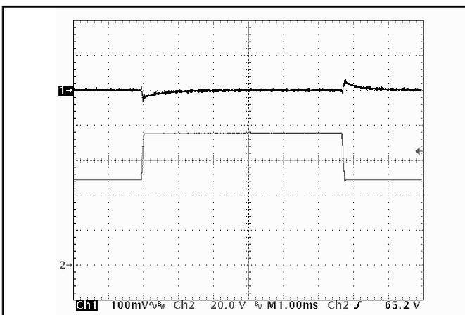
**Figure 17:** Output voltage response to step-change in input voltage ( $48\ \text{V}$  to  $75\ \text{V}$ ), at  $45\ \text{A}$  load current. Load cap:  $10\ \mu\text{F}$  tantalum capacitor and  $1\ \mu\text{F}$  ceramic cap. Ch 1:  $V_{out}$  ( $100\text{mV}/\text{div}$ ), Ch 2:  $V_{in}$  ( $20\text{V}/\text{div}$ ).
