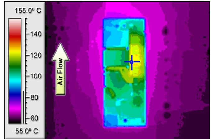
**Figure 8:** Thermal plot of converter at 35.6 a load current (53.4 W) with 70°C air flowing at the rate of 200 LFM. Air is flowing across the converter from input to output (nominal input voltage).
