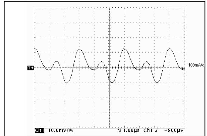
**Figure 14:** Input Terminal Ripple Current,  $i_c$ , at full rated output current and nominal input voltage with  $10\ \mu\text{H}$  source impedance and  $47\ \mu\text{F}$  electrolytic capacitor ( $50\ \text{mA}/\text{div}$ ). See Figure 13.
