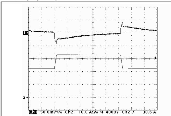
**Figure 11:** Output voltage response to step-change in load current (50%-75%-50% of  $I_{out(max)}$ );  $di/dt = 0.15A/\mu s$ . Load cap: 10  $\mu$ F, 100 m $\Omega$  ESR tantalum cap and 1  $\mu$ F ceramic cap. Ch 1: Vout (100mV/div), Ch 2: Iout (20A/div).
