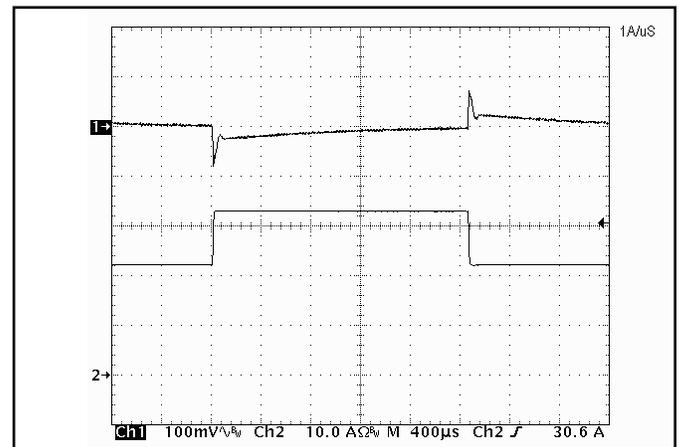
**Figure 12:** Output voltage response to step-change in load current (50%-75%-50% of  $I_{out(max)}$ );  $di/dt = 0.5A/\mu s$ . Load cap: 470  $\mu$ F, 30 m $\Omega$  ESR tantalum cap and 1  $\mu$ F ceramic cap. Ch 1: Vout (200mV/div), Ch 2: Iout (20A/div).
