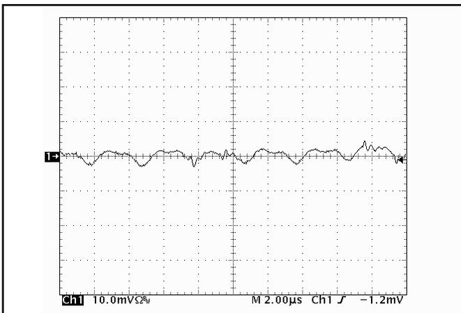
**Figure 15:** Input reflected ripple current,  $i_s$ , through a  $10\ \mu\text{H}$  source inductor, using a  $47\ \mu\text{F}$  electrolytic input capacitor ( $5\text{mA}/\text{div}$ ). See Figure 13.
