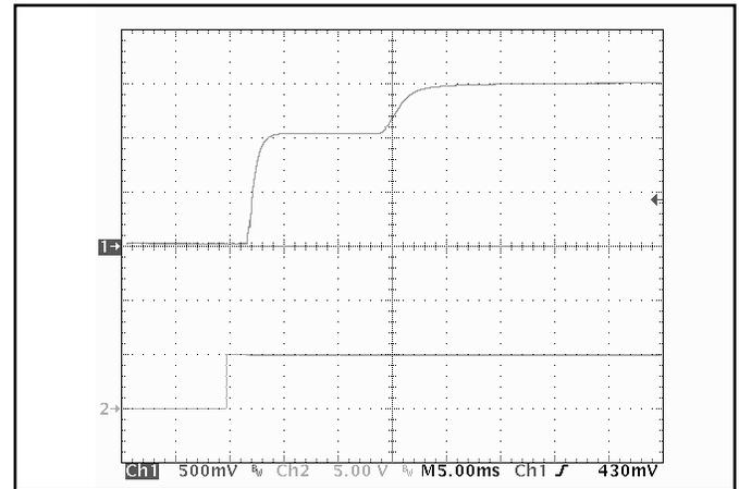
**Figure 10:** Turn-on transient at zero load (5 ms/div). Load cap: 10  $\mu$ F, 100 m $\Omega$  ESR tantalum capacitor and 1  $\mu$ F ceramic capacitor. Ch 1: Vout (500 mV/div), Ch 2: ON/OFF input (5 V/div).
