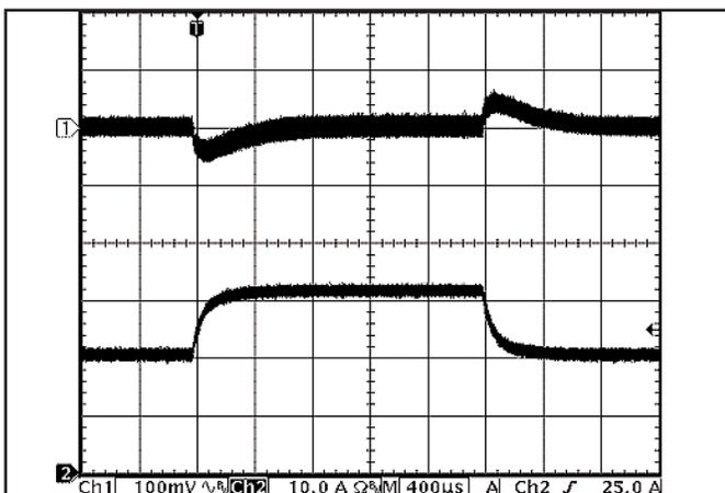
Figure 11: Output voltage response to step-change in load current (50%-75%-50% of  $I_{out(max)}$ ;  $dI/dt = 0.1A/\mu s$ ). Load cap: 10µF, 100 mΩ ESR tantalum capacitor and 1µF ceramic capacitor: Ch 1:  $V_{out}$  (100mV/div), Ch 2:  $I_{out}$  (10A/div).
