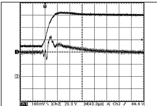
**Figure 17:** Output voltage response to step-change in input voltage ( $50\text{V}$  to  $100\text{V}$  in  $40\ \mu\text{s}$ ). Load cap:  $10\ \mu\text{F}$ ,  $100\ \text{m}\Omega$  ESR tantalum capacitor and  $1\ \mu\text{F}$  ceramic cap. Ch 1:  $V_{out}$  ( $100\text{mV}/\text{div}$ ), Ch 2:  $V_{in}$  ( $20\text{V}/\text{div}$ ).
