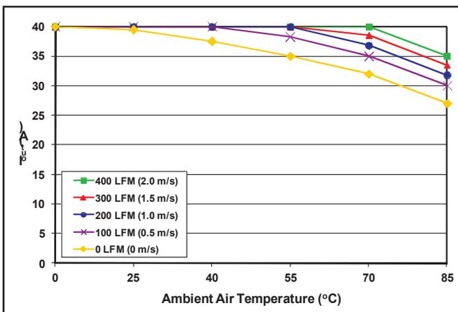
**Figure 5:** Maximum output power derating curves vs. ambient air temperature for airflow rates of 0 LFM through 400 LFM with air flowing across the converter from pin 3 to pin 1 (nominal input voltage).
