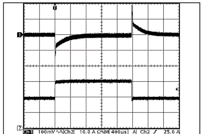
Figure 12: Output voltage response to step-change in load current (50%-75%-50% of  $I_{out(max)}$ ;  $dI/dt = 1A/\mu s$ ). Load cap: 470µF, 30 mΩ ESR tantalum capacitor and 1µF ceramic cap. Ch 1:  $V_{out}$  (100mV/div), Ch 2:  $I_{out}$  (10A/div).
