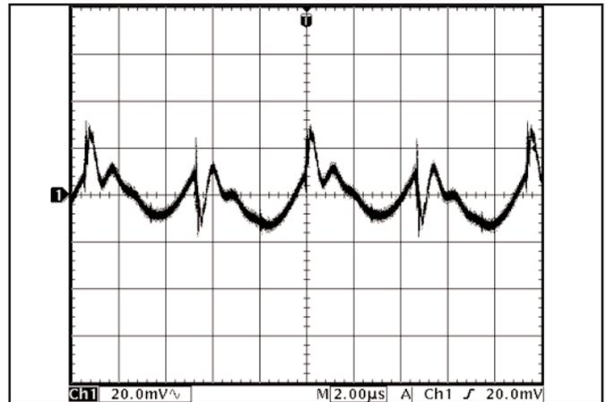
**Figure 16:** Output voltage ripple at nominal input voltage and rated load current ( $20\ \text{mV}/\text{div}$ ). Load capacitance:  $1\ \mu\text{F}$  ceramic capacitor and  $10\ \mu\text{F}$  tantalum capacitor. Bandwidth:  $500\ \text{MHz}$ . See Figure 13.
