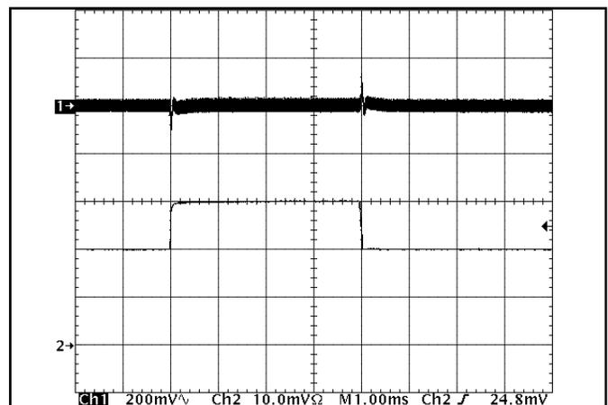
**Figure 12:** Output voltage response to step-change in load current (50%-75%-50% of I<sub>out</sub>(max); dI/dt = 5A/μs). Load cap: 480μF, 15 mΩ ESR tantalum capacitor and 1μF ceramic capacitor. Top trace: V<sub>out</sub> (200mV/div), Bottom trace: I<sub>out</sub> (20A/div).
