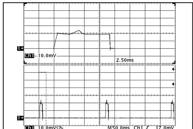
**Figure 18:** Load current ( $50\ \text{A}/\text{div}$ ) as a function of time when the converter attempts to turn on into a  $1\ \text{m}\Omega$  short circuit. Top trace ( $2.5\ \text{ms}/\text{div}$ ) is an expansion of the on-time portion of the bottom trace.
