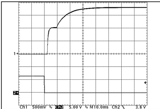
**Figure 9:** Turn-on transient at full load (resistive load) (10 ms/div). Input voltage pre-applied. Top Trace: V<sub>out</sub> (500mV/div). Bottom Trace: ON/OFF input (5V/div)
