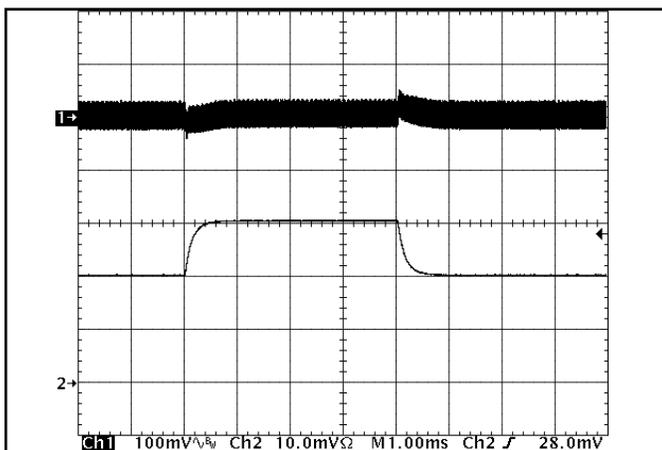
**Figure 11:** Output voltage response to step-change in load current (50%-75%-50% of I<sub>out</sub>(max); dI/dt = 0.1A/μs). Load cap: 15μF, 450 mΩ ESR tantalum capacitor and 1μF ceramic capacitor. Top trace: V<sub>out</sub> (100mV/div), Bottom trace: I<sub>out</sub> (20A/div).
