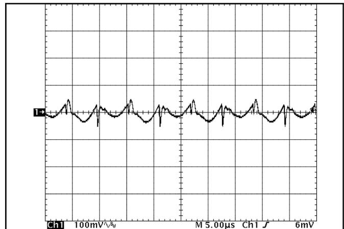
**Figure 16:** Output voltage ripple at nominal input voltage and rated load current ( $100\ \text{mV}/\text{div}$ ). Load capacitance:  $1\ \mu\text{F}$  ceramic capacitor and  $15\ \mu\text{F}$  tantalum capacitor. Bandwidth:  $20\ \text{MHz}$ . (See Figure 13)
