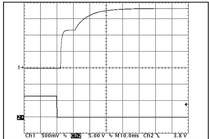
**Figure 10:** Turn-on transient at zero load (10 ms/div). Top Trace: V<sub>out</sub> (500mV/div). Bottom Trace: ON/OFF input (5V/div)
