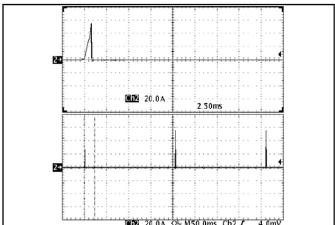
**Figure 18:** Load current ( $20\ \text{A}/\text{div}$ ) as a function of time when the converter attempts to turn on into a  $10\ \text{m}\Omega$  short circuit. Top trace ( $2.5\ \text{ms}/\text{div}$ ) is an expansion of the on-time portion of the bottom trace.
