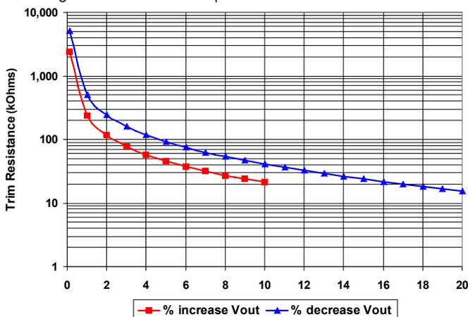
Figure C: Trim Graph for 1.8V<sub>out</sub> module
