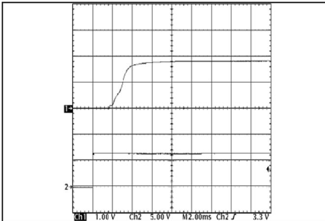
Figure 9: Turn-on transient at full load (resistive load) (2 ms/div).
