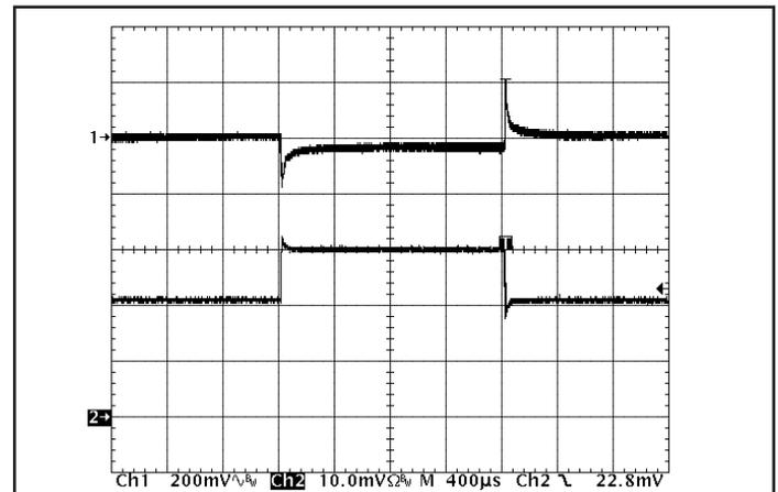
Figure 12: Output voltage response to step-change in load current (50%-75%-50% of  $I_{out(max)}$ ;  $dI/dt = 5 \text{ A}/\mu\text{s}$ ). Load cap: 470  $\mu\text{F}$ , 30 m $\Omega$  ESR tantalum capacitor and 1  $\mu\text{F}$  cermaic capacitor. Ch 1:  $V_{out}$  (200 mV/div). Ch 2:  $I_{out}$  (5 A/div).
