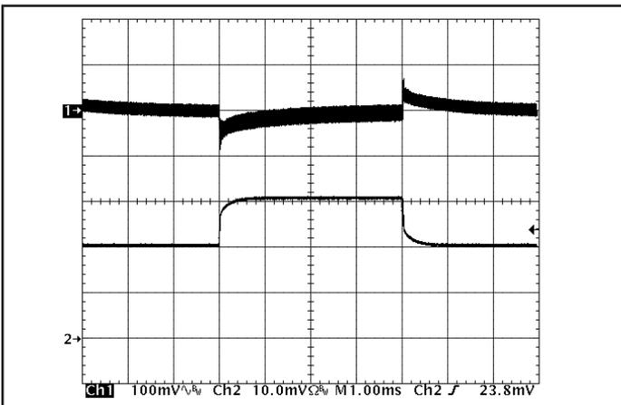
Figure 11: Output voltage response to step-change in load current (50%-75%-50% of  $I_{out(max)}$ ;  $dI/dt = 0.1 \text{ A}/\mu\text{s}$ ). Load cap: 10  $\mu\text{F}$ , 100 m $\Omega$  ESR tantalum capacitor and 1  $\mu\text{F}$  cermaic capacitor. Ch 1:  $V_{out}$  (100 mV/div). Ch 2:  $I_{out}$  (5 A/div).
