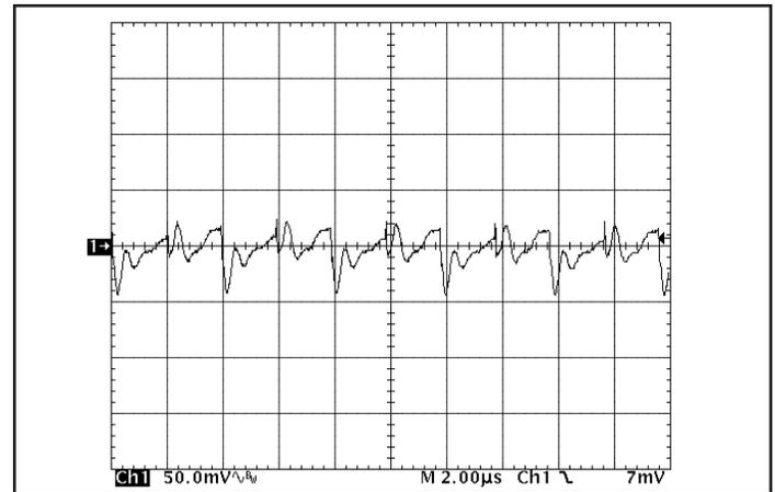
Figure 16: Output voltage ripple at nominal input voltage and rated load current ( $50\text{mV}/\text{div}$ ). Load capacitance:  $1\mu\text{F}$  ceramic capacitor and  $10\mu\text{F}$  tantalum capacitor. Bandwidth:  $20\text{MHz}$ . See Figure 13.
