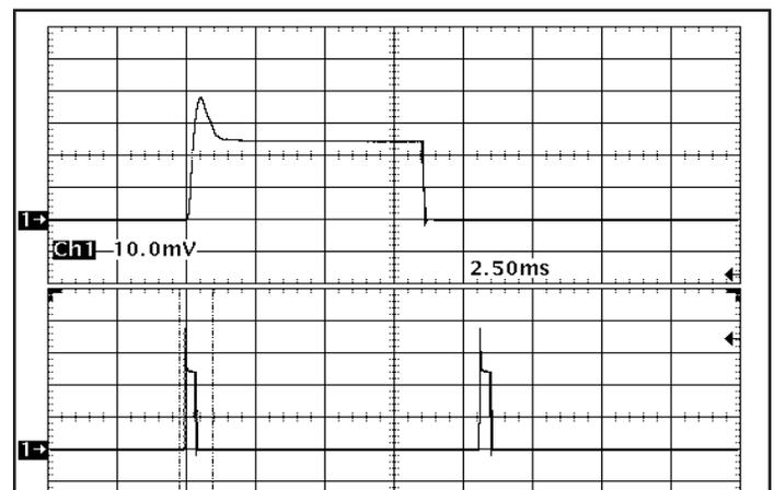
Figure 18: Load current ( $10\text{A}/\text{div}$ ) as a function of time when the converter attempts to turn on into a  $10\text{m}\Omega$  short circuit. Top trace ( $2.5\text{ms}/\text{div}$ ) is an expansion of the on-time portion of the bottom trace.
