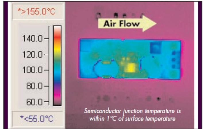
Figure 8: Thermal plot of converter at 19 amp load current with 55°C air flowing at the rate of 200 LFM. Air is flowing across the converter from input to output (nominal input voltage).
