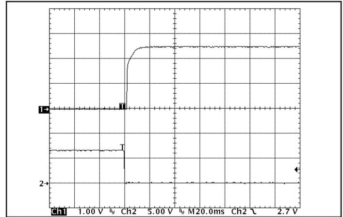
Figure 10: Turn-on transient at zero load (10 ms/div).
