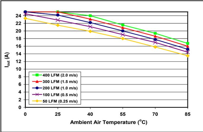
Figure 7: Maximum output power derating curves vs. ambient air temperature for airflow rates of 50 LFM through 400 LFM with air flowing lengthwise from pin 3 to pin 1 (nominal input voltage).
