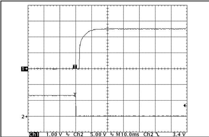
Figure 9: Turn-on transient at full load (10 ms/div).
