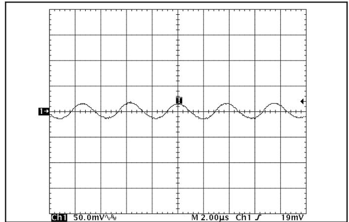
Figure 14: Input Terminal Ripple Current,  $i_c$ , at full rated output current and nominal input voltage with  $10\mu H$  source impedance and  $47\mu F$  electrolytic capacitor (200mA/div). (See Figure 13).
