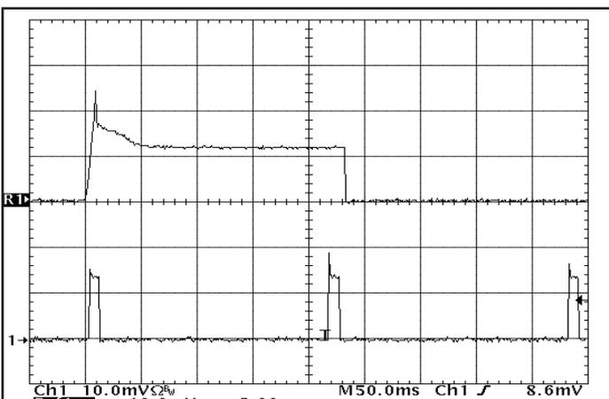
Figure 17: Load current (20A/div) as a function of time when the converter attempts to turn on into a  $10m\Omega$  short circuit. Top trace (2.0ms/div) is an expansion of the on-time portion of the bottom trace.
