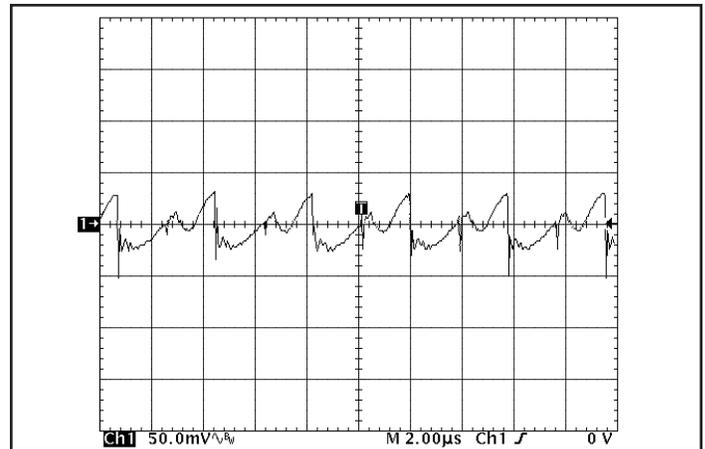
Figure 16: Output voltage ripple at nominal input voltage and rated load current (50mV/div). Load capacitance: one  $1.0\mu F$  ceramic capacitor and one  $10\mu F$  electrolytic capacitor. Bandwidth: 20 MHz. (See Figure 13).
