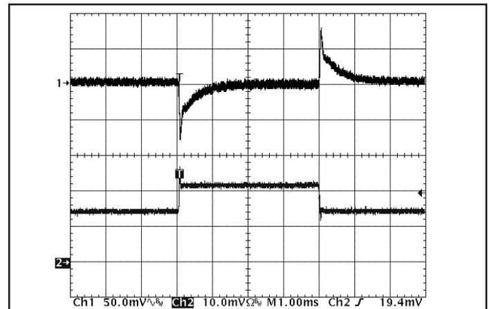
Figure 12: Output voltage response to step-change in load current (50%-75%-50% of  $I_{out(max)}$ ;  $dI/dt = 5\text{A}/\mu\text{s}$ ). Load cap: 470 $\mu\text{F}$  30 m $\Omega$  ESR tantalum cap and 1 $\mu\text{F}$  ceramic cap. Ch 1:  $V_{out}$  (50mV/div), Ch 2:  $I_{out}$  (10A/div).
