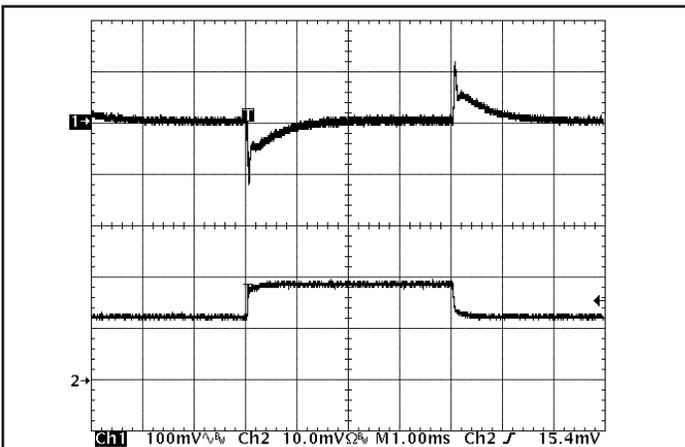
Figure 11: Output voltage response to step-change in load current (50%-75%-50% of  $I_{out(max)}$ ;  $dI/dt = 0.1\text{A}/\mu\text{s}$ ). Load cap: 100 $\mu\text{F}$  100 m $\Omega$  ESR tantalum cap and 1 $\mu\text{F}$  ceramic cap. Ch 1:  $V_{out}$  (100mV/div), Ch 2:  $I_{out}$  (10A/div).
