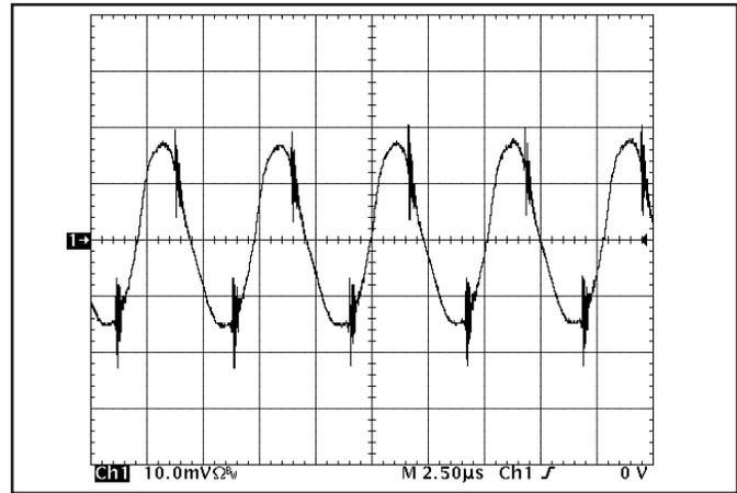
**Figure 14:** Input Terminal Ripple Current,  $i_c$ , at full rated output current and nominal input voltage with  $10\ \mu\text{H}$  source impedance and  $47\ \mu\text{F}$  electrolytic capacitor (200 mA/div). (See Figure 13)
