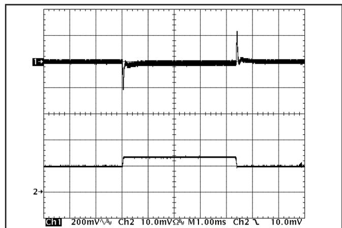
**Figure 12:** Output voltage response to step-change in load current (50%-75%-50% of I<sub>out</sub>(max); dI/dt = 5A/μs). Load cap: 480μF, 15 mΩ ESR tantalum cap and 1μF ceramic cap. Top trace: V<sub>out</sub> (200mV/div), Bottom trace: I<sub>out</sub> (50A/div).
