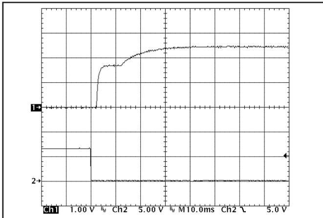
**Figure 9:** Turn-on transient at full load (resistive load) (10 ms/div). Input voltage pre-applied. Top Trace: V<sub>out</sub> (1V/div). Bottom Trace: ON/OFF input (5V/div)
