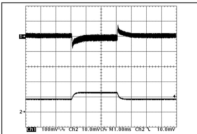
**Figure 11:** Output voltage response to step-change in load current (50%-75%-50% of I<sub>out</sub>(max); dI/dt = 0.1A/μs). Load cap: 15μF, 450 mΩ ESR tantalum cap and 1μF ceramic cap. Top trace: V<sub>out</sub> (100mV/div), Bottom trace: I<sub>out</sub> (50A/div).
