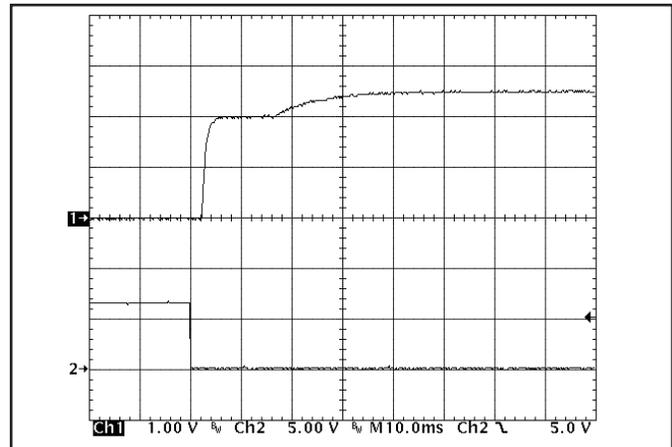
**Figure 10:** Turn-on transient at zero load (10 ms/div). Top Trace: V<sub>out</sub> (1V/div) Bottom Trace: ON/OFF input (5V/div)
