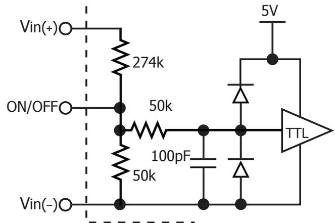
Figure B: Internal ON/OFF pin circuitry
