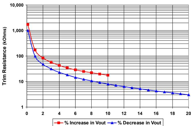
**Figure C: Trim Graph for 3.3V<sub>out</sub> module**
