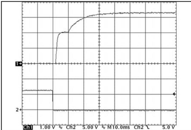
Figure 9: Turn-on transient at full load (resistive load) (10 ms/div).
