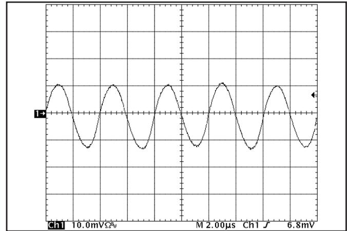
**Figure 14:** Input Terminal Ripple Current,  $i_c$ , at full rated output current and nominal input voltage with  $10\ \mu\text{H}$  source impedance and  $47\ \mu\text{F}$  electrolytic capacitor ( $200\ \text{mA}/\text{div}$ ). See Figure 13.
