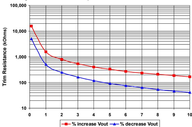
Figure C: Trim Graph for 5.0V<sub>out</sub> module
