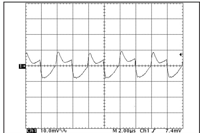
**Figure 16:** Output voltage ripple at nominal input voltage and rated load current ( $20\ \text{mV}/\text{div}$ ). Load capacitance:  $1\ \mu\text{F}$  ceramic capacitor and  $10\ \mu\text{F}$  tantalum capacitor. Bandwidth:  $20\ \text{MHz}$ . See Figure 13.
