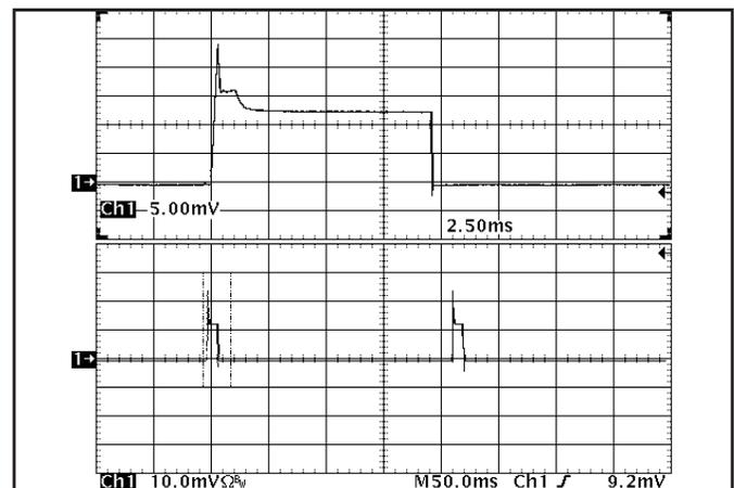
**Figure 18:** Load current ( $5\ \text{A}/\text{div}$ ) as a function of time when the converter attempts to turn on into a  $10\ \text{m}\Omega$  short circuit. Top trace ( $2.5\ \text{ms}/\text{div}$ ) is an expansion of the on-time portion of the bottom trace.
