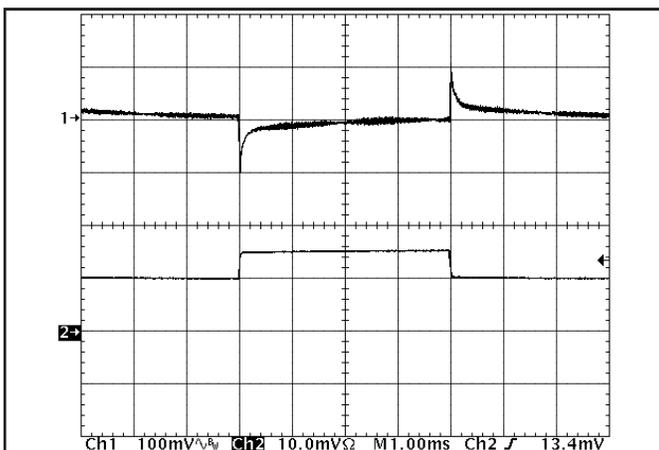
Figure 11: Output voltage response to step-change in load current (50%-75%-50% of I<sub>out</sub>(max); dI/dt = 0.1A/μs). Load cap: 10μF, 100 mΩ ESR tantalum capacitor and 1μF ceramic capacitor. Ch 1: V<sub>out</sub> (100mV/div), Ch 2: I<sub>out</sub> (5A/div).
