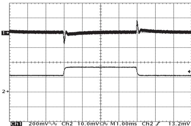
Figure 11: Output voltage response to step-change in load current (50%-75%-50% of  $I_{out(max)}$ ;  $dI/dt = 0.1\text{A}/\mu\text{s}$ ). Load cap: 15 $\mu\text{F}$ , 450mOhm ERS tantalum cap and 1 $\mu\text{F}$  ceramic cap. Top trace:  $V_{out}$  (200mV/div). Bottom trace:  $I_{out}$  (20A/div).
