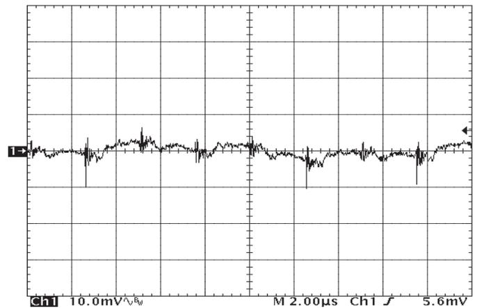
Figure 16: Output voltage ripple at nominal input voltage and rated load current ( $10\ \text{mV}/\text{div}$ ). Load capacitance:  $1\ \mu\text{F}$  ceramic capacitor and one  $15\ \mu\text{F}$  tantalum capacitor. Bandwidth:  $20\ \text{MHz}$ . (See Figure 13).
