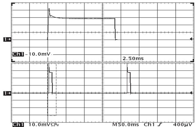
Figure 18: Load current ( $20\text{A}/\text{div}$ ) as a function of time when the converter attempts to turn on into a  $1\ \text{m}\Omega$  short circuit. Top trace ( $2.5\text{ms}/\text{div}$ ) is an expansion of the on-time portion of the bottom trace.
