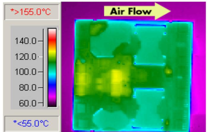
Figure 6: Thermal plot of converter at 39A load current (195W) with 55°C air flowing at the rate of 200 LFM. Air is flowing from input to output (nominal input voltage).
