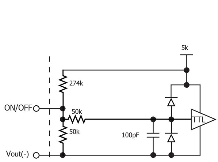
Figure B: Internal ON/OFF pin circuitry
