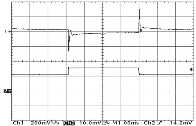
Figure 12: Output voltage response to step-change in load current (50%-75%-50% of  $I_{out(max)}$ ;  $dI/dt = 5\text{A}/\mu\text{s}$ ). Load cap: 470 $\mu\text{F}$ , 15mOhm ESR tantalum cap and 1 $\mu\text{F}$  ceramic cap. Top trace:  $V_{out}$  (200mV/div). Bottom trace:  $I_{out}$  (20A/div).
