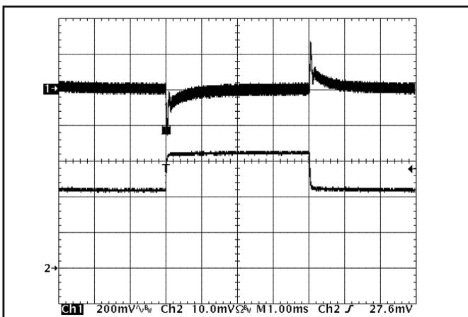
**Figure 11:** Output voltage response to step-change in load current (50%-75%-50% of I<sub>out</sub>(max); dI/dt = 0.1A/μs). Load cap: 10μF, 100 mΩ ESR tantalum capacitor and 1μF ceramic capacitor. Ch 1: V<sub>out</sub> (200mV/div), Ch 2: I<sub>out</sub> (1A/div).
