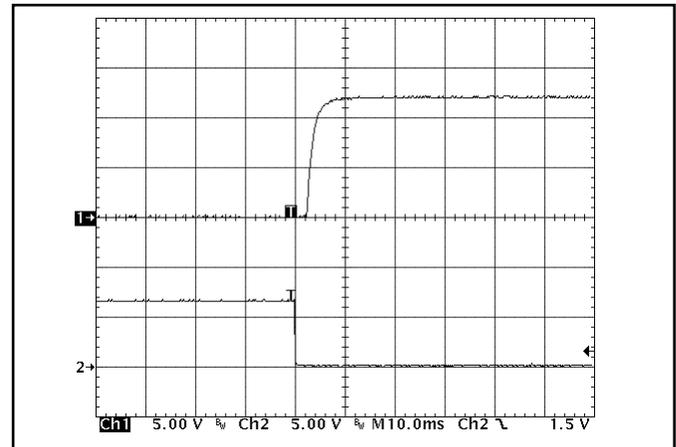
**Figure 10:** Turn-on transient at zero load (10 ms/div). Ch 1: V<sub>out</sub> (5V/div); Ch 2: ON/OFF input (5V/div)
