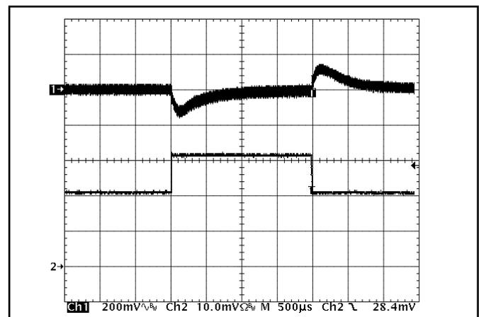
**Figure 12:** Output voltage response to step-change in load current (50%-75%-50% of I<sub>out</sub>(max); dI/dt = 5A/μs). Load cap: 470μF, 30 mΩ ESR tantalum capacitor and 1μF ceramic cap. Ch 1: V<sub>out</sub> (200mV/div), Ch 2: I<sub>out</sub> (1A/div).
