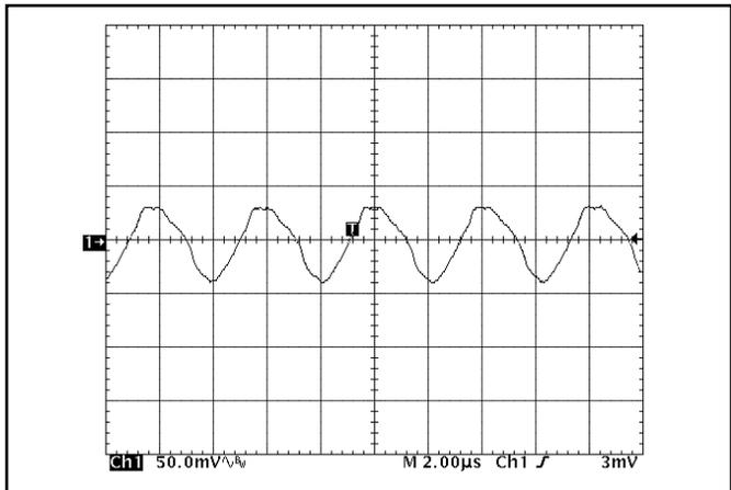
**Figure 16:** Output voltage ripple at nominal input voltage and rated load current ( $50\ \text{mV}/\text{div}$ ). Load capacitance:  $1\ \mu\text{F}$  ceramic capacitor and  $10\ \mu\text{F}$  tantalum capacitor. Bandwidth:  $20\ \text{MHz}$ . See Figure 13.
