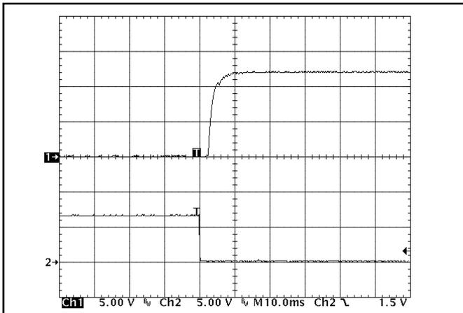
**Figure 9:** Turn-on transient at full load (resistive load) (10 ms/div). Input voltage pre-applied. Ch 1: V<sub>out</sub> (5V/div); Ch 2: ON/OFF input (5V/div)
