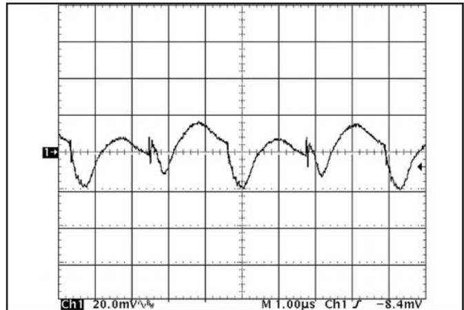
**Figure 16:** Output voltage ripple at nominal input voltage and rated load current (20 mV/div). Load capacitance:  $1\ \mu\text{F}$  ceramic capacitor and  $15\ \mu\text{F}$  tantalum capacitor. Bandwidth: 20 MHz. (See Figure 13)
