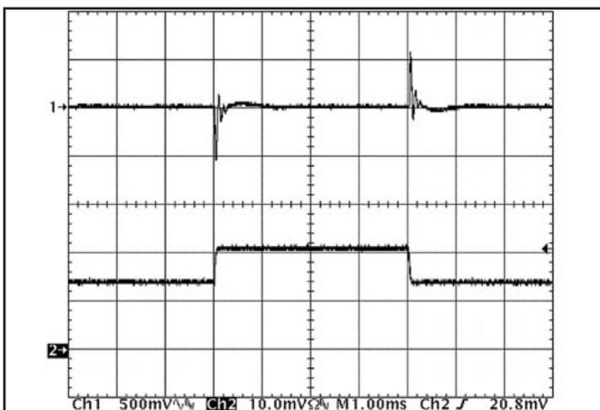
Figure 11: Output voltage response to step-change in load current (50%-75%-50% of I<sub>out</sub>(max); dI/dt = 0.1A/μs). Load cap: 15μF, 450 mΩ ESR tantalum capacitor and 1μF ceramic capacitor. Top trace: V<sub>out</sub> (500mV/div), Bottom trace: I<sub>out</sub> (5A/div).
