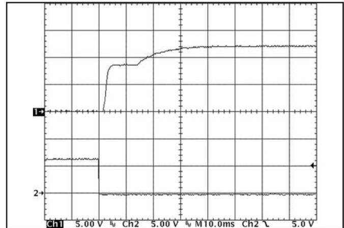
Figure 10: Turn-on transient at zero load (10 ms/div). Top Trace: V<sub>out</sub> (5V/div) Bottom Trace: ON/OFF input (5V/div)
