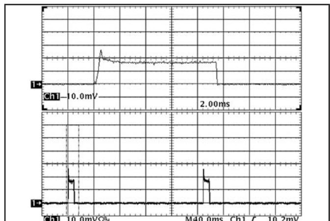
**Figure 18:** Load current (10A/div) as a function of time when the converter attempts to turn on into a  $1\ \text{m}\Omega$  short circuit. Top trace (2ms/div) is an expansion of the on-time portion of the bottom trace.
