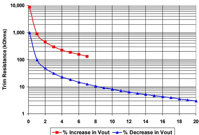
Figure C: Trim Graph for 12V<sub>out</sub> module
