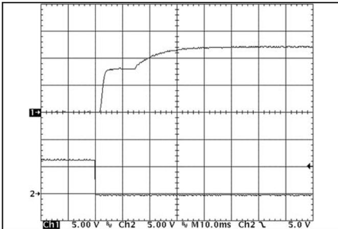
Figure 9: Turn-on transient at full load (resistive load) (10 ms/div). Input voltage pre-applied. Top Trace: V<sub>out</sub> (5V/div). Bottom Trace: ON/OFF input (5V/div)
