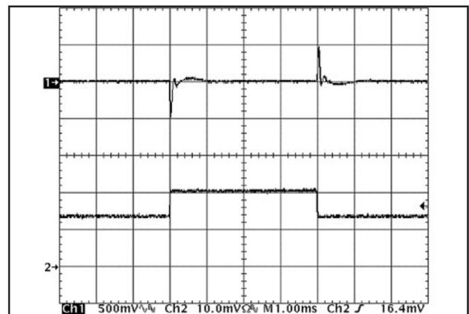
Figure 12: Output voltage response to step-change in load current (50%-75%-50% of I<sub>out</sub>(max); dI/dt = 5A/μs). Load cap: 480μF, 15 mΩ ESR tantalum capacitor and 1μF ceramic capacitor. Top trace: V<sub>out</sub> (500mV/div), Bottom trace: I<sub>out</sub> (5A/div).
