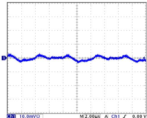
Figure 13: Input reflected ripple current, is, through a 4.7µH source inductor, using a 100µF input capacitor, at nominal input voltage and rated load current (10mA/div). See Figure 11.
