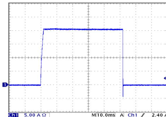
Figure 16: Load current (5A/div) as a function of time when the converter attempts to turn on into a 10 mW short circuit.
