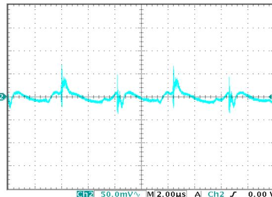
Figure 14: Output voltage ripple at nominal input voltage and rated load current (50mV/div). Load capacitance: 1µF ceramic capacitor and 10µF tantalum capacitor. Bandwidth: 500 MHz. See Figure 11.
