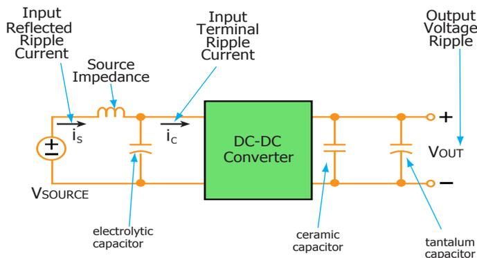
Figure 11: Test set-up diagram showing measurement points for Input Terminal Ripple Current (Figure 12), Input Reflected Ripple Current (Figure 13) and Output Voltage Ripple (Figure 14).
