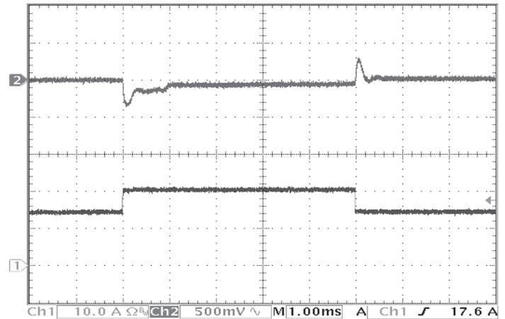
Figure 10: Output voltage response to step-change in load current (50%-75%-50% of  $I_{out(max)}$ ;  $dI/dt = 5A/\mu s$ ). Load cap: 470uF, 15 m $\Omega$  ESR tantalum capacitor. Top trace: Vout (500mV/div), Bottom trace: Iout (10A/div).
