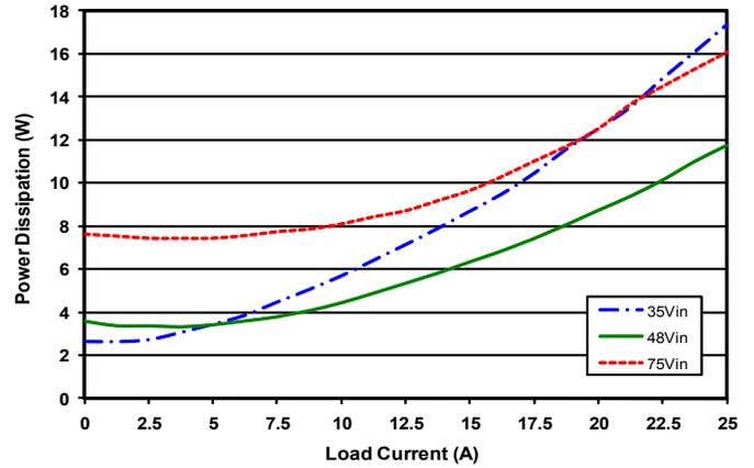
Figure 2: Power dissipation at nominal output voltage vs. load current for minimum, nominal, and maximum input voltage at 25°C.
