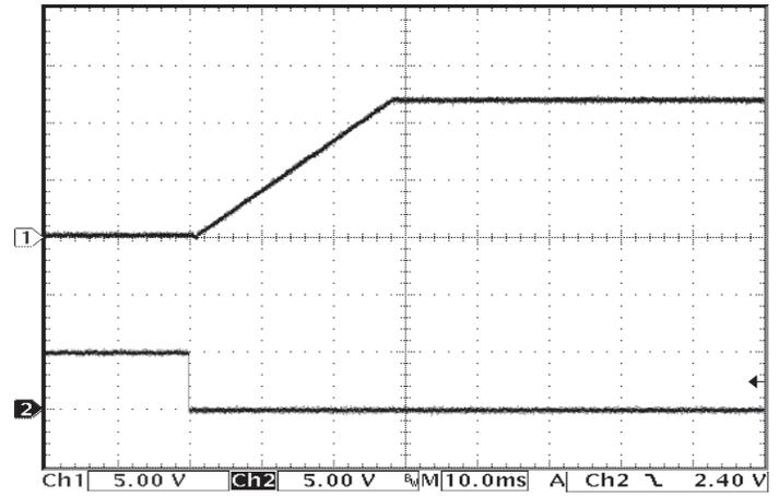
Figure 8: Turn-on transient at zero load (10 ms/div).
