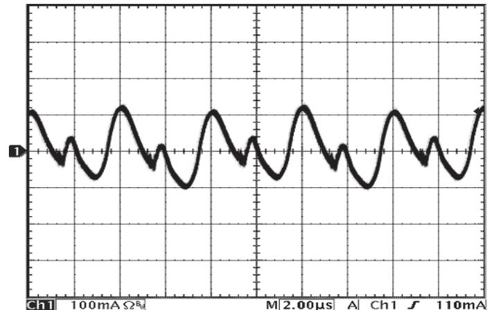
Figure 12: Input Terminal Ripple Current,  $i_c$ , at full rated output current and nominal input voltage with 4.7uH source impedance and 100uF electrolytic capacitor (100 mA/div). See Figure 11.
