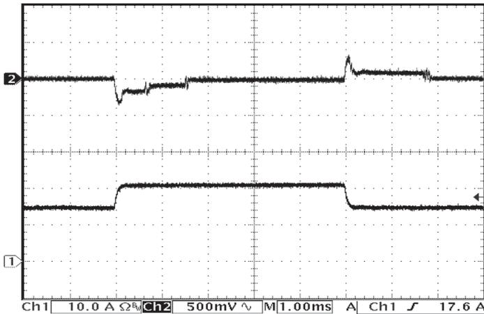
Figure 9: Output voltage response to step-change in load current (50%-75%-50% of  $I_{out(max)}$ ;  $dI/dt = 0.1A/\mu s$ ). Load cap: 1uF ceramic and 10uF tantalum capacitors. Top trace: Vout (500mV/div), Bottom trace: Iout (10A/div).
