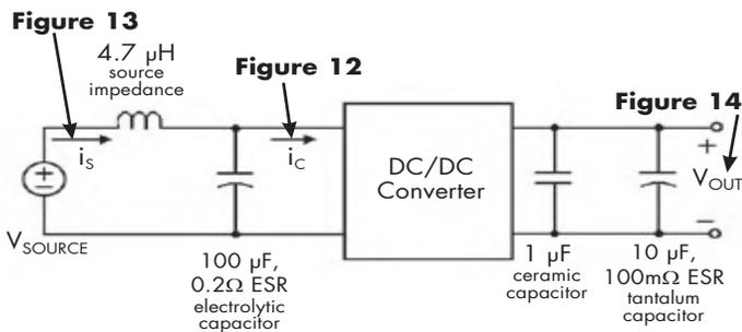
Figure 11: Test set-up diagram showing measurement points for Input Terminal Ripple Current (Fig 12), Input Reflected Ripple Current (Fig 13) and Output Voltage Ripple (Fig 14).
