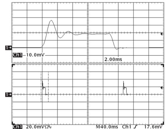
Figure 18: Load current (5A/div) as a function of time when the converter attempts to turn on into a  $1 m\Omega$  short circuit. Top trace (2ms/div) is an expansion of the on-time portion of the bottom trace.
