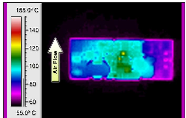
Figure 6: Thermal plot of converter at 3 amp load current (72 W) with 55°C air flowing at the rate of 200 LFM. Air is flowing across the converter from pin 3 to pin 1 (nominal input voltage).
