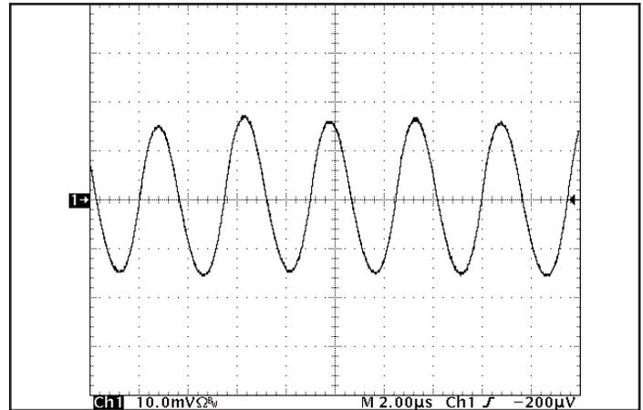
Figure 14: Input Terminal Ripple Current,  $i_c$ , at full rated output current and nominal input voltage with  $10\mu\text{H}$  source impedance and  $47\mu\text{F}$  electrolytic capacitor (200 mA/div). See Figure 13.
