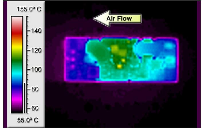
Figure 8: Thermal plot of converter at 3 amp load current (72 W) with 55°C air flowing at the rate of 200 LFM. Air is flowing across the converter from input to output (nominal input voltage).
