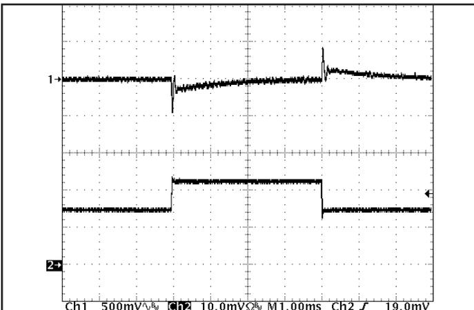
Figure 11: Output voltage response to step-change in load current (50%-75%-50% of  $I_{out(max)}$ ;  $di/dt = 0.1 A/\mu s$ ). Load cap: 15  $\mu F$ , 100 m $\Omega$  ESR tantalum cap and 1  $\mu F$  ceramic cap. Ch 1: Vout (500 mV/div). Ch 2: Iout (1 A/div).
