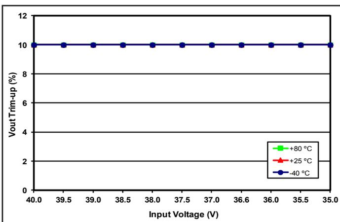
Figure 23: Achievable trim-up percentage vs. input voltage. at +85°C, +25°C and -40°C (all at full load).
