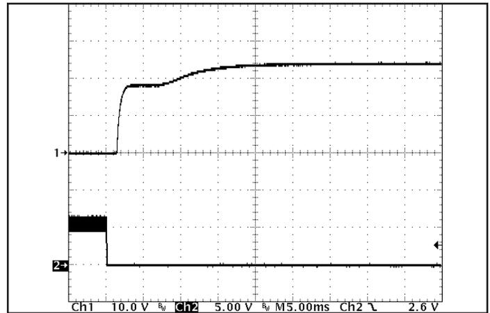
Figure 10: Turn-on transient at zero load (5 ms/div). Ch 1: Vout (10 mV/div). Ch 2: ON/OFF input (5 V/div)
