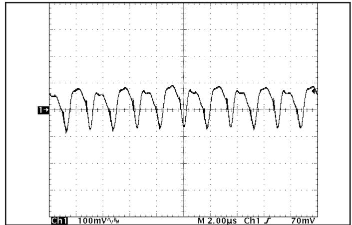
Figure 16: Output voltage ripple at nominal input voltage and rated load current (100 mV/div). Load capacitance:  $1\mu\text{F}$  ceramic capacitor and one  $15\mu\text{F}$  tantalum capacitor. Bandwidth: 20 MHz. See Figure 13.
