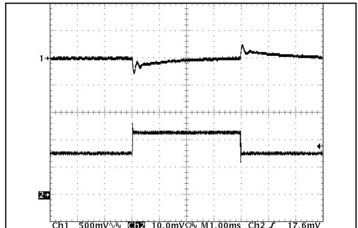
Figure 12: Output voltage response to step-change in load current (50%-75%-50% of  $I_{out(max)}$ ;  $di/dt = 1 A/\mu s$ ). Load cap: 90  $\mu F$ , 15  $\mu F$ , 100 m $\Omega$  ESR tantalum cap and 1  $\mu F$  ceramic cap. Ch 1: Vout (500 mV/div). Ch 2: Iout (1 A/div).
