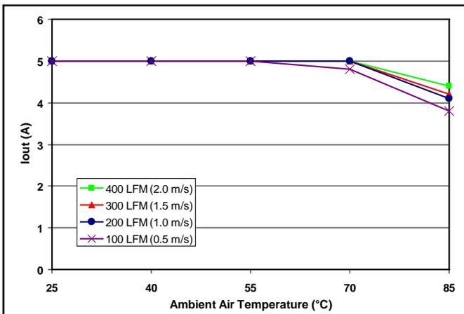
**Figure 5:** Maximum output power derating curves vs. ambient air temperature for airflow rates of 100 LFM through 400 LFM with air flowing across the converter from input to output (nominal input voltage).
