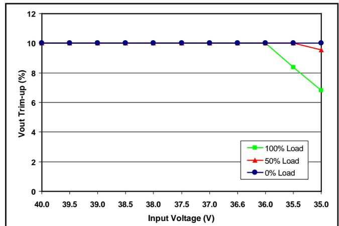
**Figure 12:** Percentage of output voltage trim-up that can be achieved at various input voltages from V<sub>in</sub> 35V-40V and output loads of 0%, 50% and full load.
