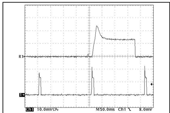
**Figure 18:** Load current (5A/div) as a function of time when the converter attempts to turn on into a  $1\ \text{m}\Omega$  short circuit. Top trace (2.5ms/div) is an expansion of the on-time portion of the bottom trace.
