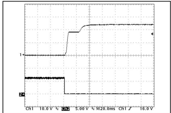
**Figure 10:** Turn-on transient at zero load current (20 ms/div). Ch 1: V<sub>out</sub> (10V/div). Ch 2: ON/OFF input (5V/div)
