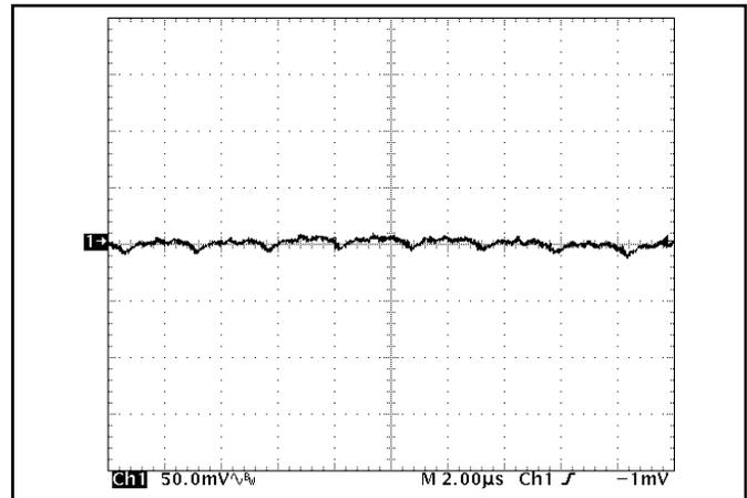
**Figure 16:** Output voltage ripple at nominal input voltage and rated load current (50 mV/div). Load capacitance:  $1\ \mu\text{F}$  ceramic capacitor and  $10\ \mu\text{F}$  tantalum capacitor. Bandwidth: 20 MHz. See Figure 13.
