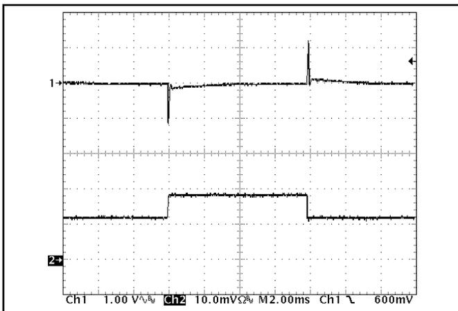
**Figure 11:** Output voltage response to step-change in load current (50%-75%-50% of I<sub>out</sub>(max); dI/dt = 0.1A/µs). Load cap: 10µF, 100 mΩ ESR tantalum capacitor and 1µF ceramic capacitor. Ch 1: V<sub>out</sub> (1V/div), Ch 2: I<sub>out</sub> (2A/div).
