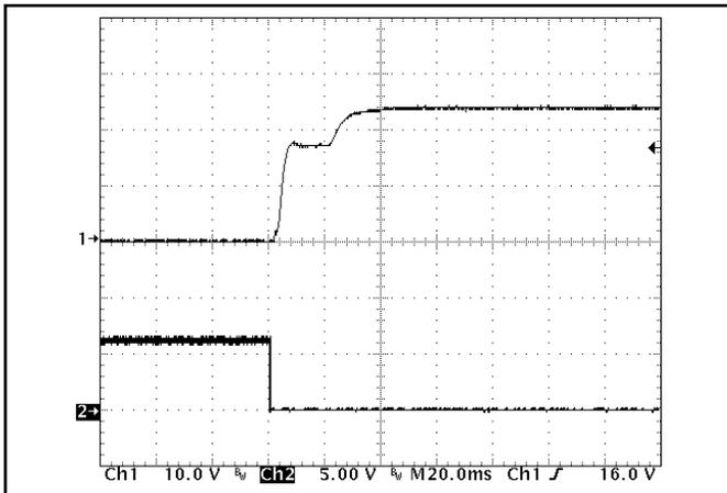
**Figure 9:** Turn-on transient at full rated load (resistive load) (20 ms/div) Input voltage pre-applied. Ch 1: V<sub>out</sub> (10V/div). Ch 2: ON/OFF input (5V/div)
