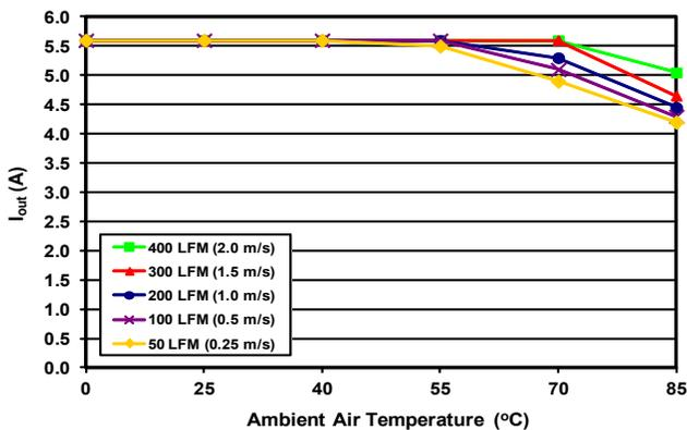
Figure 5: Maximum output power derating curves vs. ambient air temperature for airflow rates of 50 LFM through 400 LFM with air flowing across the converter from pin 1 to pin 3 (nominal input voltage).
