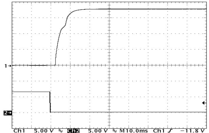
Figure 10: Turn-on transient at zero load (10 ms/div). Ch 1: Vout (5V/div). Ch 2: ON/OFF input (5V/div)
