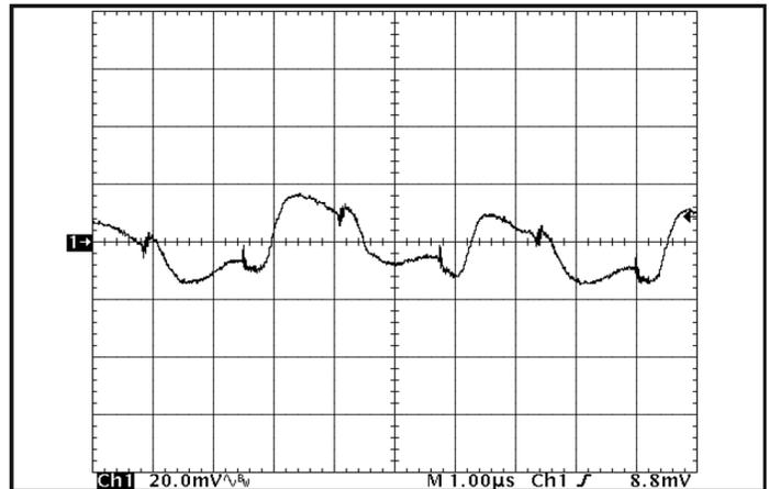
**Figure 16:** Output voltage ripple at nominal input voltage and rated load current ( $20\ \text{mV}/\text{div}$ ). Load capacitance:  $1\ \mu\text{F}$  ceramic capacitor and  $10\ \mu\text{F}$  tantalum capacitor. Bandwidth: 20 MHz. See Figure 13.
