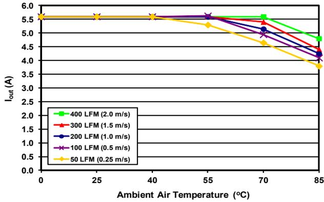
Figure 7: Maximum output power-de-rating curves vs. ambient air temperature for airflow rates of 50 LFM through 400 LFM with air flowing lengthwise from input to output (nominal input voltage).
