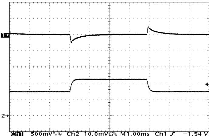
Figure 11: Output voltage response to step-change in load current (50%-75%-50% of Iout(max); dI/dt = 0.1A/μs). Load cap: 10μF, 100 mΩ ESR tantalum capacitor and 1μF ceramic capacitor. Ch 1: Vout (500mV/div), Ch 2: Iout (2A/div).
