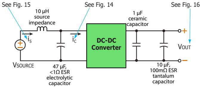
**Figure 13:** Test set-up diagram showing measurement points for Input Terminal Ripple Current (Figure 14), Input Reflected Ripple Current (Figure 15) and Output Voltage Ripple (Figure 16).
