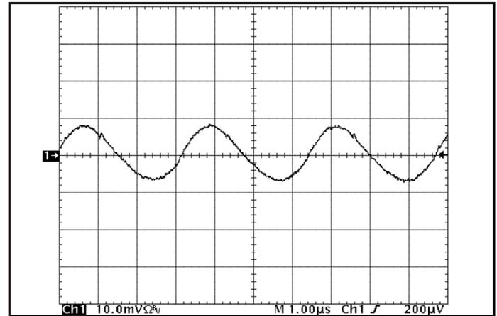
**Figure 14:** Input Terminal Ripple Current,  $i_c$ , at full rated output current and nominal input voltage with  $10\ \mu\text{H}$  source impedance and  $47\ \mu\text{F}$  electrolytic capacitor ( $100\ \text{mA}/\text{div}$ ). See Figure 13.
