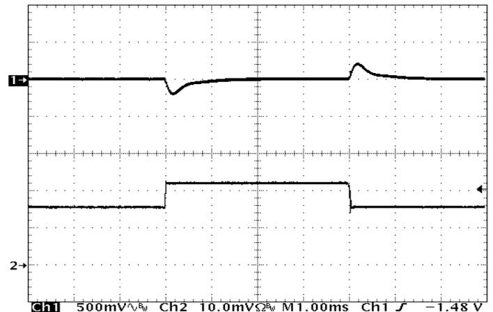
Figure 12: Output voltage response to step-change in load current (50%-75%-50% of Iout(max); dI/dt = 5A/μs). Load cap: 100μF, 30 mΩ ESR tantalum capacitor and 1μF ceramic cap. Ch 1: Vout (500mV/div), Ch 2: Iout (2A/div).
