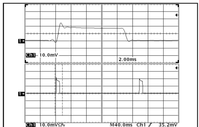
**Figure 18:** Load current ( $5\ \text{A}/\text{div}$ ) as a function of time when the converter attempts to turn on into a  $10\ \text{m}\Omega$  short circuit. Top trace ( $2.0\ \text{ms}/\text{div}$ ) is an expansion of the on-time portion of the bottom trace.
