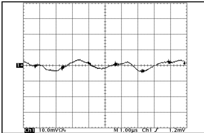
**Figure 15:** Input reflected ripple current,  $i_s$ , through a  $10\ \mu\text{H}$  source inductor at nominal input voltage and rated load current ( $5\ \text{mA}/\text{div}$ ). See Figure 13.
