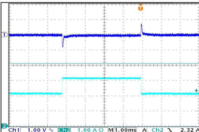
Figure 5: Output voltage response to step-change in load current (50%-75%-50% of I<sub>out</sub>(max); dI/dt = 0.1 A/μs). Load cap: 1 μF ceramic capacitor. Ch 1: V<sub>out</sub>, Ch 2: I<sub>out</sub> (1A/div.)
