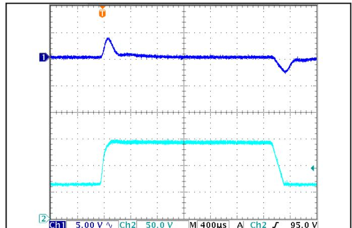
Figure 6: Output voltage response to step-change in input voltage (1000 V/ms). Load cap: 1 μF ceramic capacitor. Ch 1: V<sub>out</sub>, Ch 2: V<sub>in</sub>.
