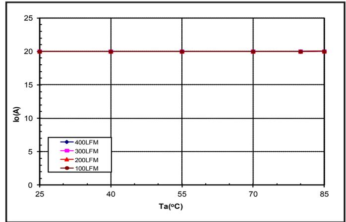
Figure 4: Encased Converter (0.9" heatsink) max. output current derating vs. ambient air temperature for airflow rates of 100 LFM through 400 LFM. Air flows across the converter from input to output (nominal input voltage).
