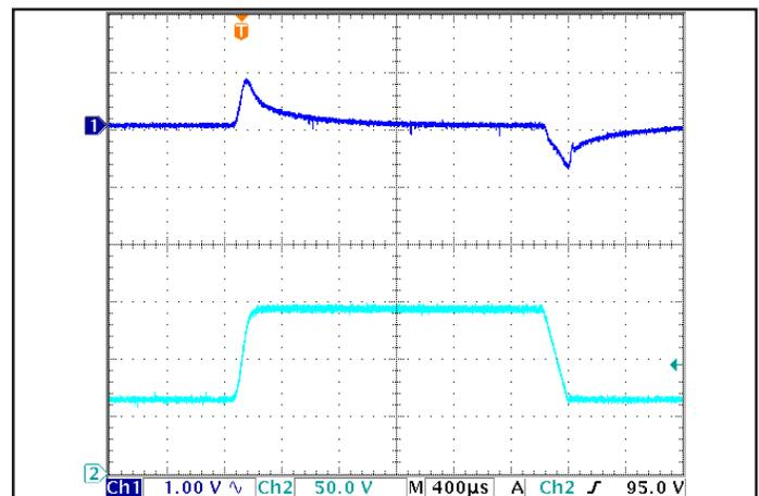
Figure 6: Output voltage response to step-change in input voltage (1V/μs). Load cap: 1 μF ceramic and 15 μF tantalum capacitors. Ch 1: V<sub>out</sub>, Ch 2: V<sub>in</sub>.
