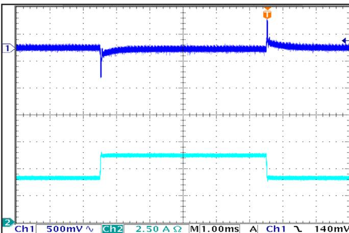
Figure 5: Output voltage response to step-change in load current (50%-75%-50% of I<sub>out</sub>(max); di/dt = 0.1 A/μs). Load cap: 1 μF ceramic and 15 μF tantalum capacitors. Ch 1: V<sub>out</sub>, Ch 2: I<sub>out</sub> (2.5A/div)
