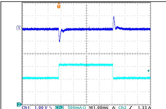
Figure 5: Output voltage response to step-change in load current (50%-75%-50% of I<sub>out</sub>(max); dI/dt = 0.1 A/μs). Load cap: 1 μF ceramic capacitor. Ch 1: V<sub>out</sub>, Ch 2: I<sub>out</sub>(0.5A/div).
