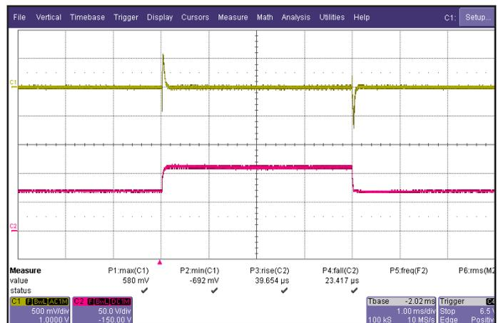
Figure 6: Output voltage and input voltage response to step-change in input voltage (1V/μs). Load cap: 1 μF ceramic and 15 μF tantalum capacitors. Ch 1: Vout, Ch 2: Vin.
