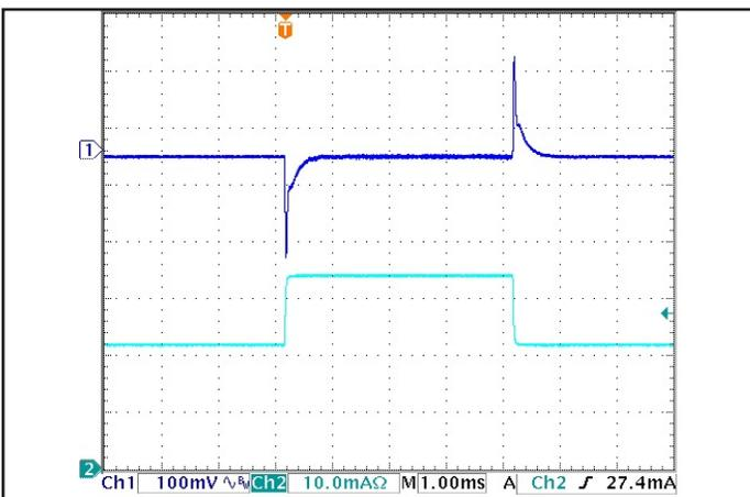
Figure 5: Output voltage response to step-change in load current (50%-75%-50% of I<sub>out</sub>(max); dI/dt = 0.1 A/μs). Load cap: 1 μF ceramic and 15 μF tantalum capacitors. Ch 1: V<sub>out</sub>, Ch 2: I<sub>out</sub>(10.0A/div).
