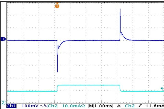
Figure 5: Output voltage response to step-change in load current (50%-75%-50% of  $I_{out(max)}$ ;  $dI/dt = 0.1 A/\mu s$ ). Load cap: 1  $\mu F$  ceramic and 15  $\mu F$  tantalum capacitors. Ch 1:  $V_{out}$ , Ch 2:  $I_{out}(5.0A/div)$ .
