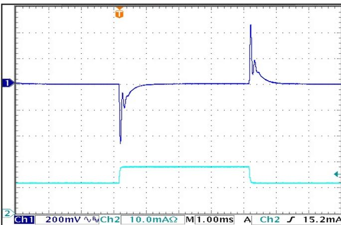
Figure 5: Output voltage response to step-change in load current (50%-75%-50% of I<sub>out</sub>(max); dI/dt = 0.1 A/μs). Load cap: 1 μF ceramic capacitor. Ch 1: V<sub>out</sub>, Ch 2: I<sub>out</sub>(2.5A/div).
