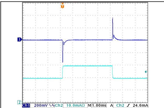
Figure 5: Output voltage response to step-change in load current (50%-75%-50% of I<sub>out</sub>(max); dI/dt = 0.1 A/μs). Load cap: 1 μF ceramic and 15 μF tantalum capacitors. Ch 1: V<sub>out</sub>, Ch 2: I<sub>out</sub>(2.0A/div).
