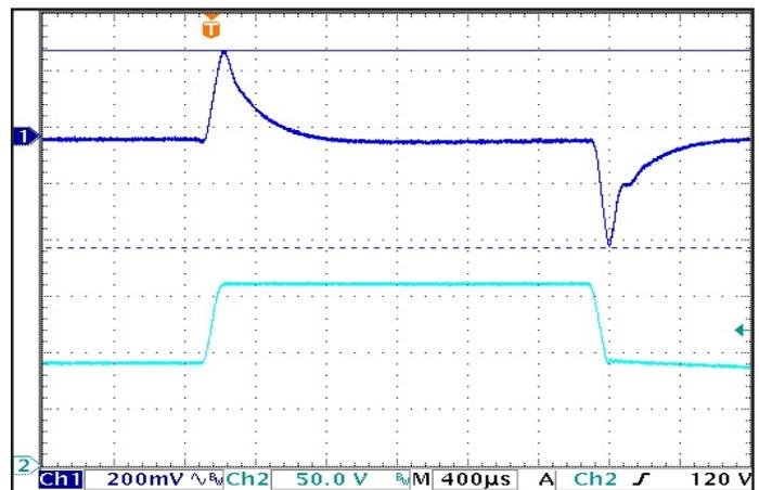
Figure 6: Output voltage response to step-change in input voltage (1V/ms). Load cap: 1 μF ceramic capacitor. Ch 1: V<sub>out</sub>, Ch 2: V<sub>in</sub>.
