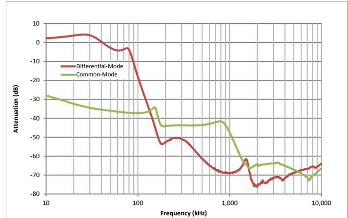
*Figure A: Typical Common Mode and Differential Mode Attenuation provided by the filter as a function of frequency. Source resistance is 50Ω.*
