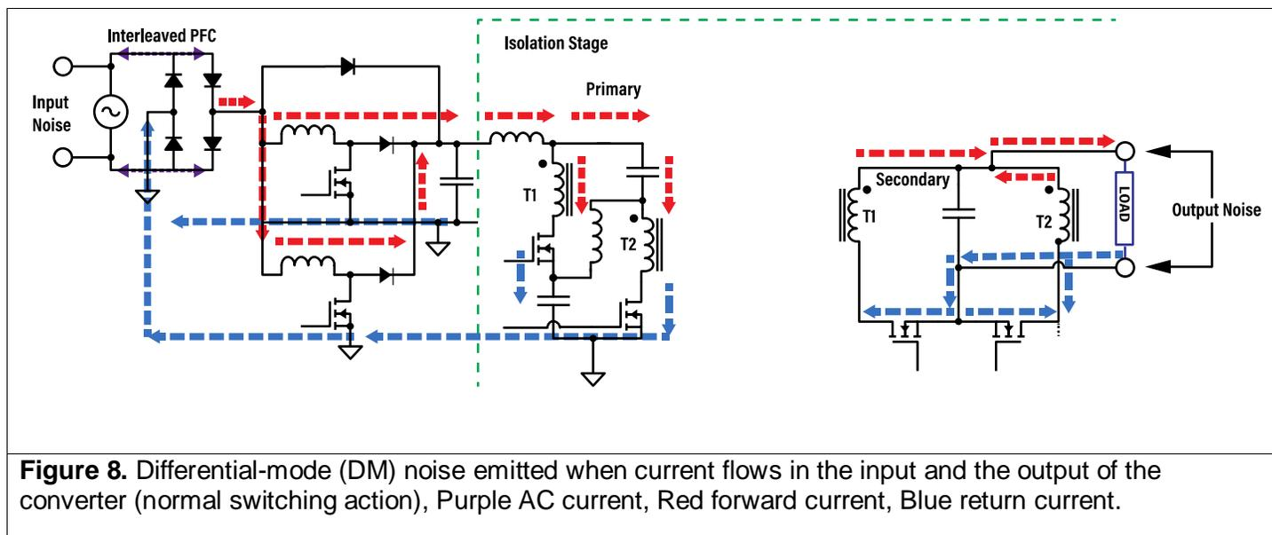
**Figure 8.** Differential-mode (DM) noise emitted when current flows in the input and the output of the converter (normal switching action), Purple AC current, Red forward current, Blue return current.
