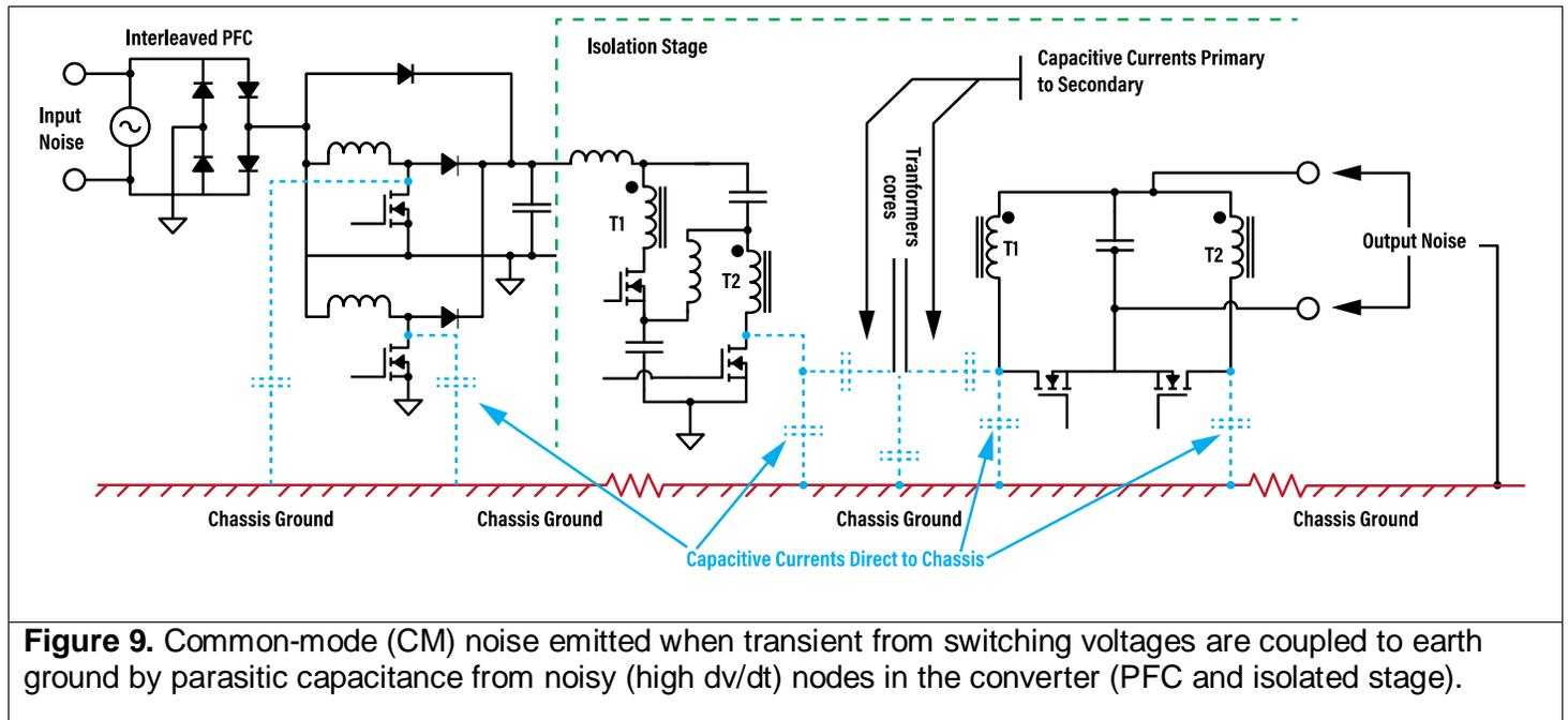
**Figure 9.** Common-mode (CM) noise emitted when transient from switching voltages are coupled to earth ground by parasitic capacitance from noisy (high  $dv/dt$ ) nodes in the converter (PFC and isolated stage).
