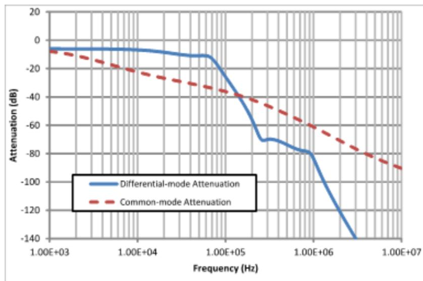
**Figure 12.** ACF-U-230-QT CM (Common-mode) and DM (Differential-mode) filter attenuation (simulated, source and load resistance are 50Ω).
