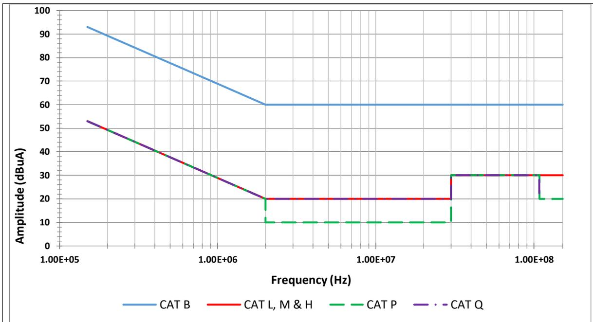
Figure 1. DO-160 Conducted Emissions Limits for Power Lines [1].
