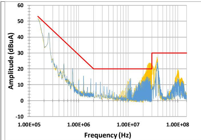
**Figure 26.** DO-160G CAT-M conducted emissions with C8 set to 10nF.
