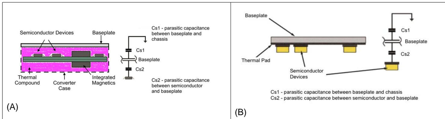
**Figure 10(A & B).** Physical design of a SynQor enclosed module (A), vs. the traditional physical design for PFC modules (B). Note the substantially lower capacitance (Cs1 & Cs2) in SynQor’s design.
