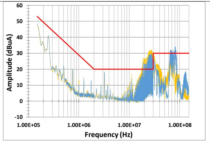
**Figure 25.** DO-160G CAT-M conducted emissions (same setup as Figure 24) with the addition of two 56nF differential capacitors placed across the input and output terminals of the filter.
