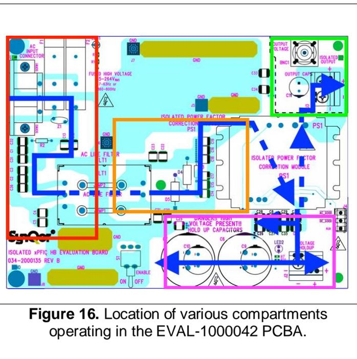
**Figure 16.** Location of various compartments operating in the EVAL-1000042 PCBA.
