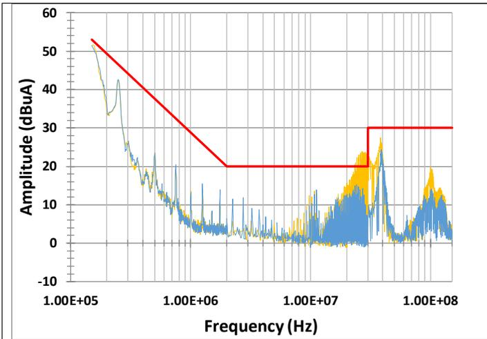
**Figure 24.** DO-160G CAT-M conducted emissions with C8 set to 10nF (Y-capacitor, input to output).
