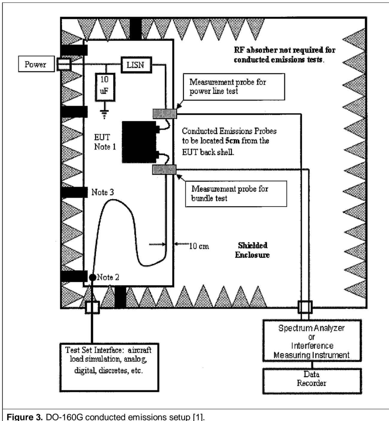
Figure 3. DO-160G conducted emissions setup [1].
