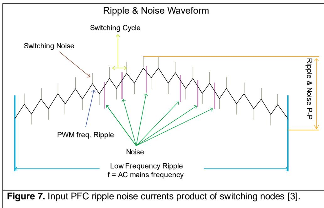
Figure 7 represents the typical input current of a PFC stage. The PFC input current ripple has the following identifiable AC components:
