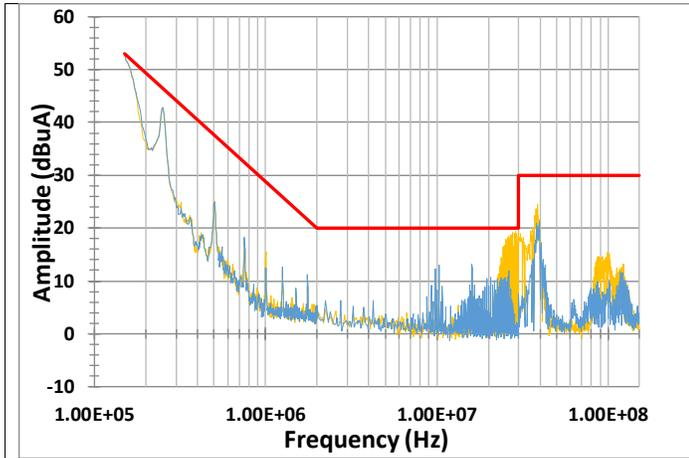
**Figure 18.** DO-160G CAT-M Grounded baseplates (filter and converter) conducted emissions (C8 capacitance 20nF). Same scan as shown in Figure 11.
