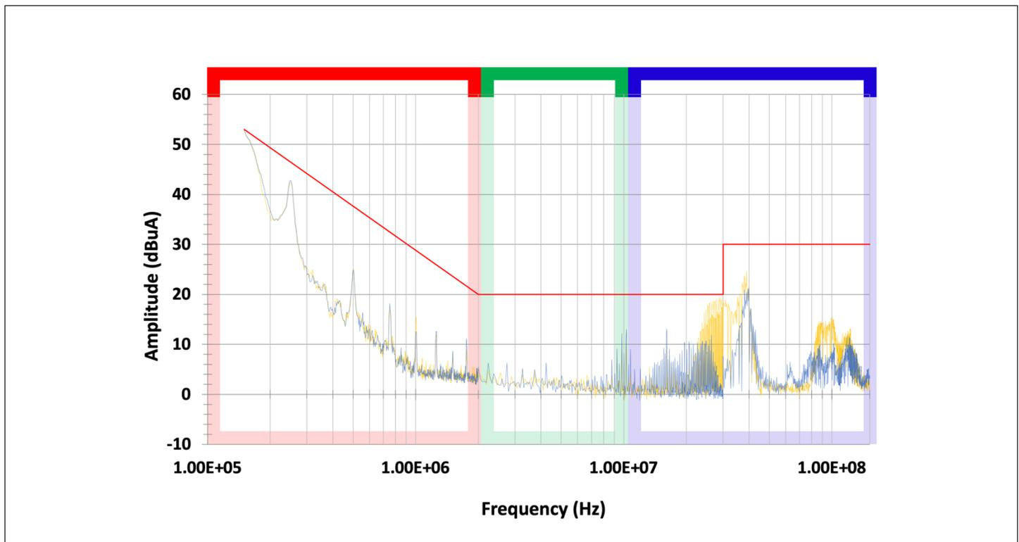
**Figure 13.** DO-160G CAT-M conducted emissions without the recommended Y-capacitors:
