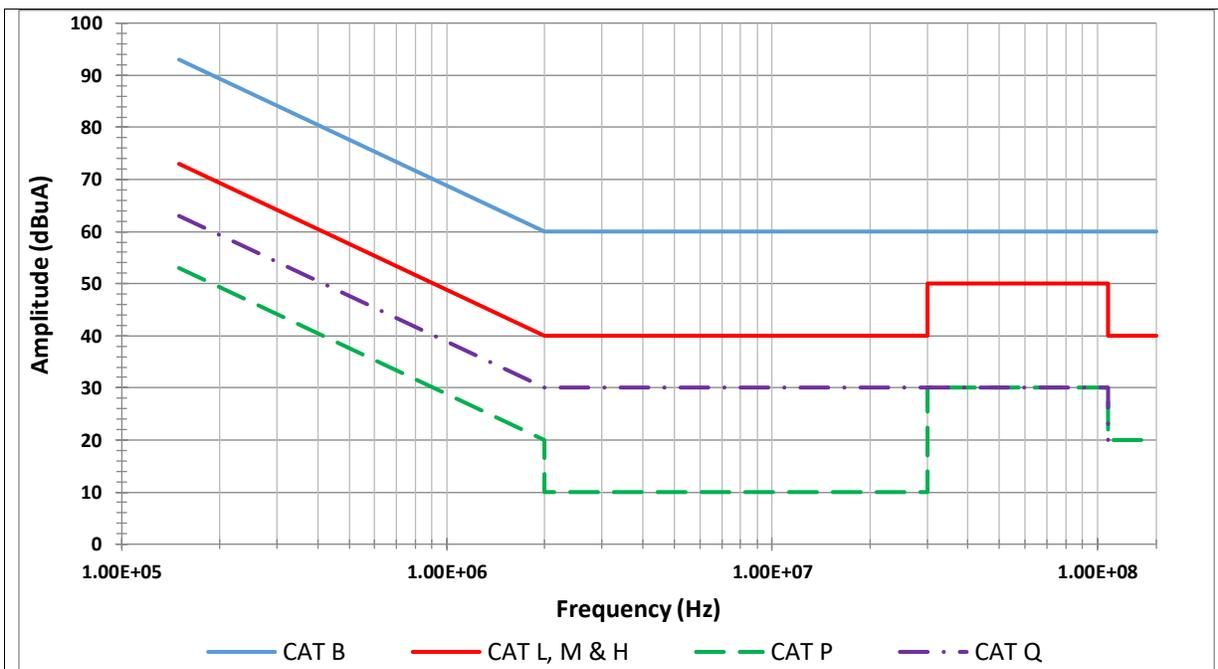
Figure 2. DO-160 Conducted Emissions Limits for Cable Bundles [1].
