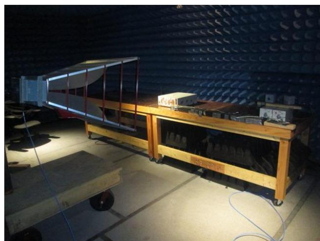
**Figure 5.** Radiated Emissions Setup.
