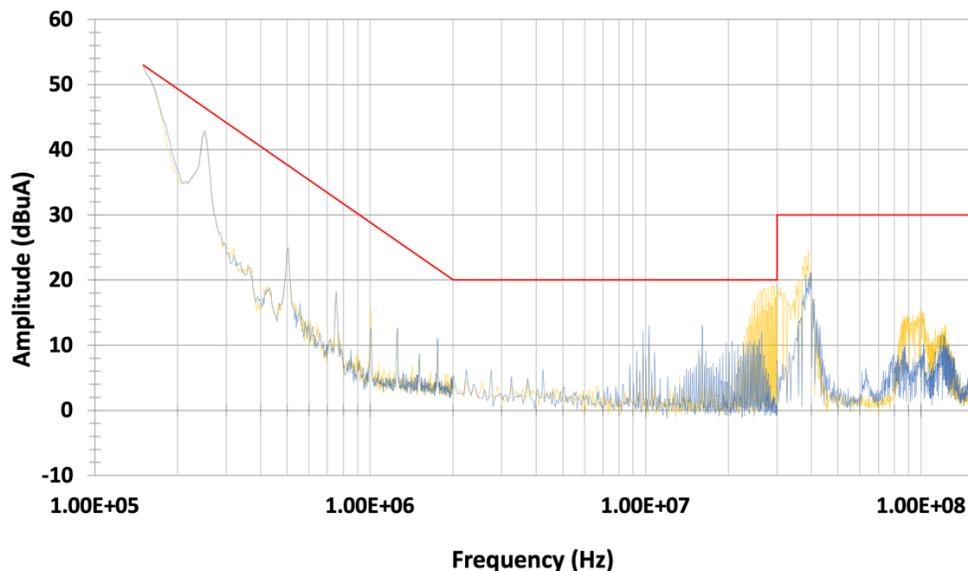
**Figure 11.** DO-160G CAT-M Grounded baseplates (filter and converter) conducted emissions. Blue: Line conducted emissions; Yellow: Neutral conducted emissions
