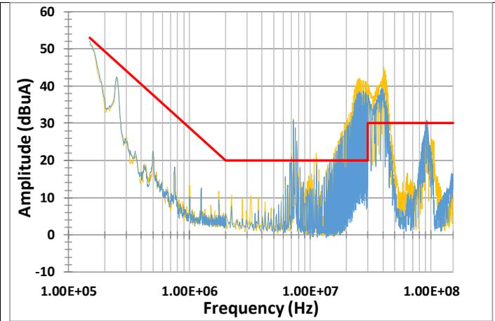
**Figure 19.** DO-160G CAT-M Ungrounded baseplates conducted emissions (C8 capacitance 20nF).
