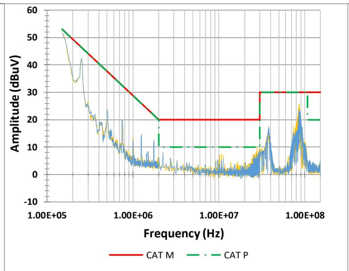
**Figure 23.** DO-160G CAT-M and CAT-P conducted emissions with C8 set to 10nF and an external common-mode choke.
