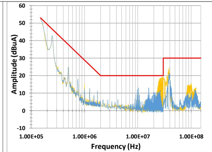
**Figure 21.** DO-160G CAT-M conducted emissions recommended C8 capacitance 20nF (grounded baseplates).
