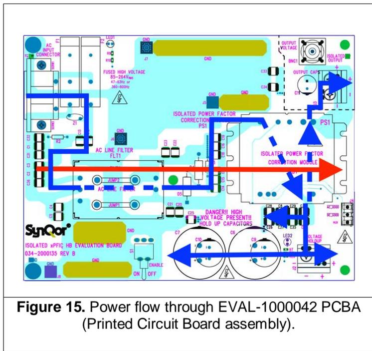
**Figure 15.** Power flow through EVAL-1000042 PCBA (Printed Circuit Board assembly).
