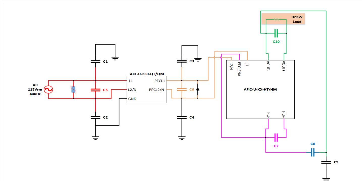
**Figure 17.** Eval-100042 evaluation board compartmental diagram (follows Figure 16 color scheme).
