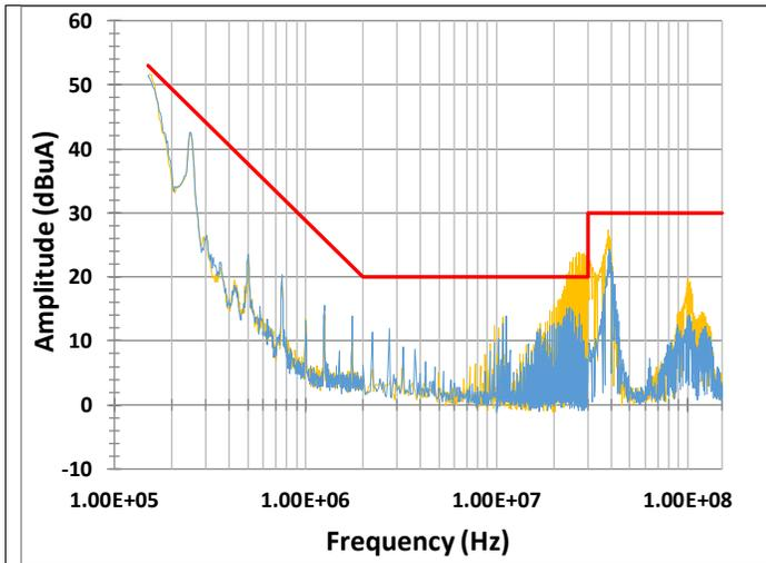
**Figure 20.** DO-160G CAT-M conducted emissions C8 set to 10nF (grounded baseplates).
