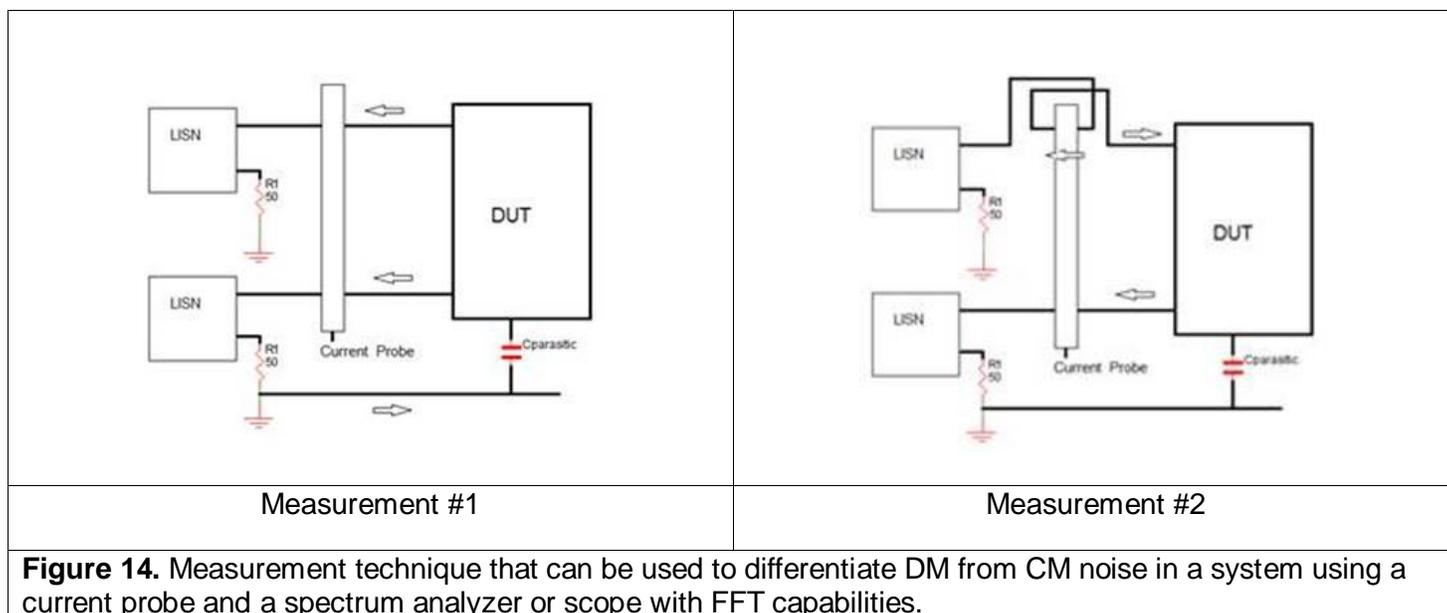
**Figure 14.** Measurement technique that can be used to differentiate DM from CM noise in a system using a current probe and a spectrum analyzer or scope with FFT capabilities.
