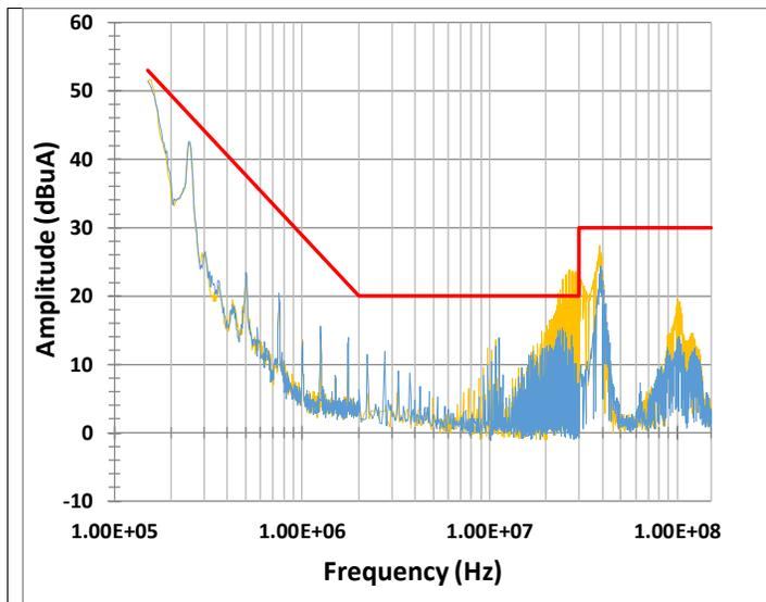
**Figure 22.** DO-160G CAT-M conducted emissions with C8 set to 10nF.
