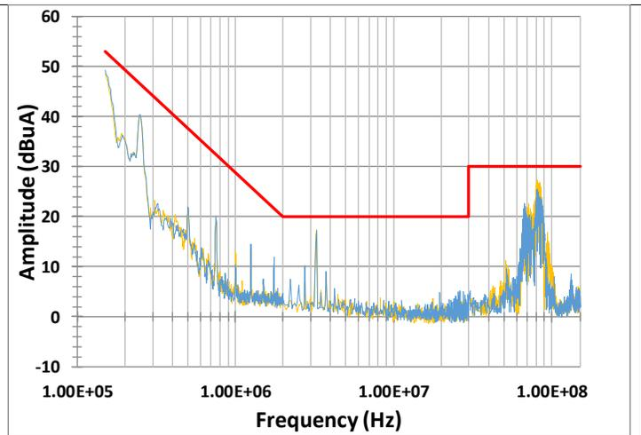
**Figure 27.** DO-160G CAT-M conducted emissions (same setup as Figure 25). CM choke added on the input, and three 56nF differential capacitors placed across the input and output terminals of the filter.
