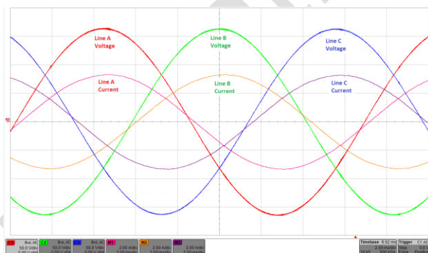
Figure 2 - 60Hz, Full Load, 5 msec/div Line Voltage: 50 V/div Line Current 2 A/div
