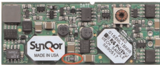
Figure 1: Photograph showing typical location of the sense resistor for Power Qor Eighth-brick product families.
