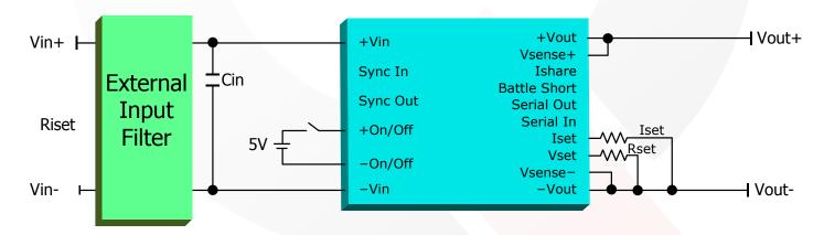
Note 1: An Input Stability calculation will need to be performed to ensure proper damping of the system. Use the SynQor application notes "Guidelines for Testing SynQor DC-DC Converters" and "Input System Instability" to cover the topics of properly testing and implementing the DC-DC converters as a load when using this evaluation board.
