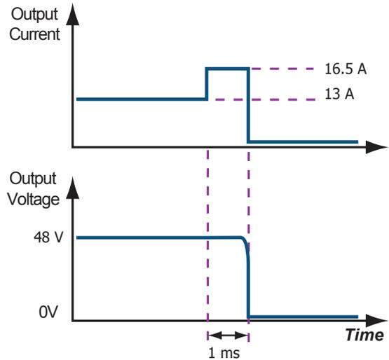
Figure C: Output Overload protection diagram (not to scale)
