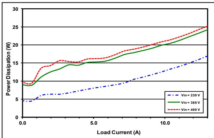
Figure 3: Power dissipation vs. load current for minimum, nominal, and maximum input voltage at T<sub>CASE</sub>=25 °C.
