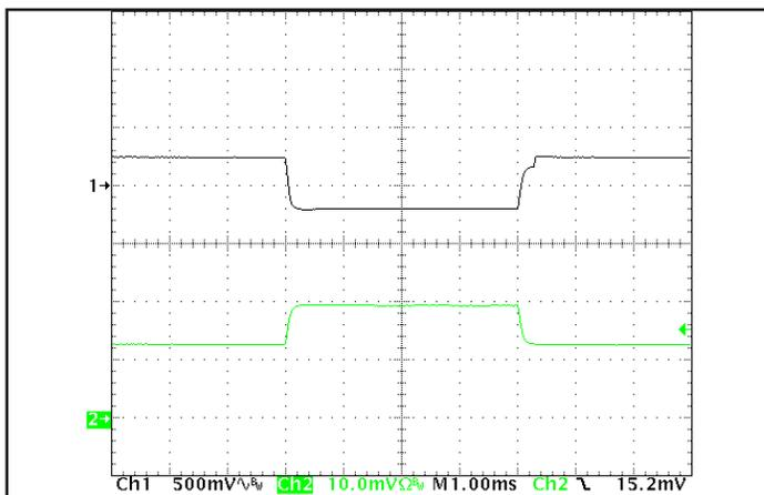
Figure 11: Output voltage response to step-change in load current (50%-75%-50% of  $I_{out(max)}$ ;  $dI/dt = 0.1$  A/ $\mu$ s). Load cap: 10  $\mu$ F tantalum cap and 1  $\mu$ F ceramic cap. Ch 1: Vout (500 mV/div), Ch 2: Iout (5 A/div).
