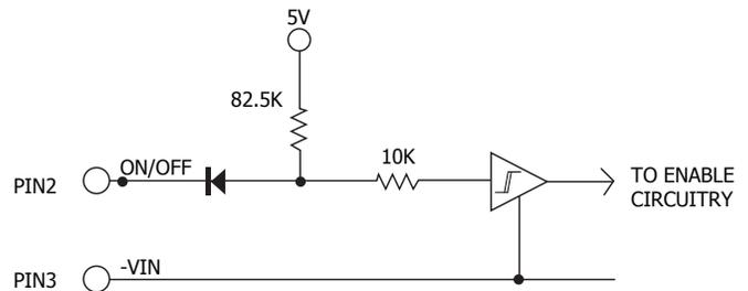
Figure B: Internal ON/OFF pin circuitry
