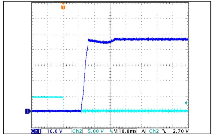
Figure 10: Turn-on transient at half load (resistive load) (10 ms/div). Load cap: 10  $\mu$ F tantalum capacitor and 500  $\mu$ F ceramic capacitor bank. Input voltage pre-applied. Ch 1: Vout (10 V/div). Ch 2: ON/OFF input (5 V/div).
