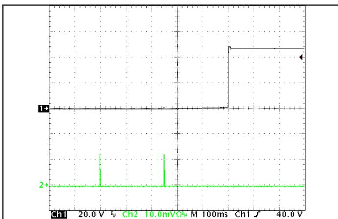
Figure 17: Rise of output voltage after the removal of a short circuit across the output terminals.  $R_{\text{short}} = 5\ \text{m}\Omega$ . Ch1:  $V_{\text{out}}$  ( $20\ \text{V}/\text{div}$ ). Ch2:  $I_{\text{out}}$  ( $50\ \text{A}/\text{div}$ ). Bandwidth:  $20\ \text{MHz}$ .
