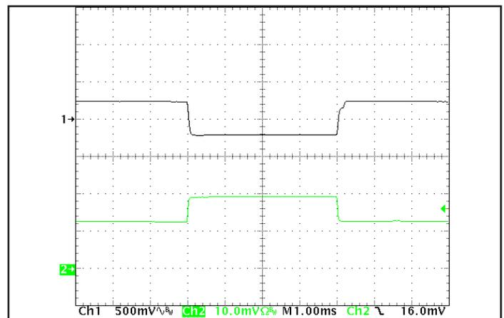
Figure 12: Output voltage response to step-change in load current (50%-75%-50% of  $I_{out(max)}$ ;  $dI/dt = 1$  A/ $\mu$ s). Load cap: 10  $\mu$ F tantalum cap and 500  $\mu$ F ceramic capacitor bank. Ch 1: Vout (500 mV/div), Ch 2: Iout (5 A/div).
