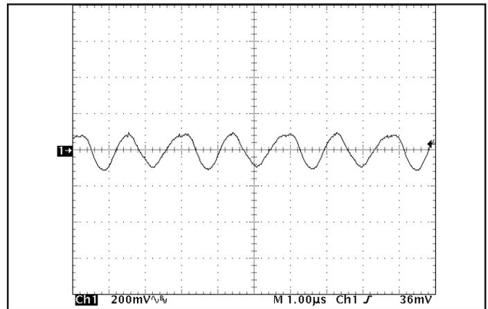
Figure 16: Output voltage ripple at nominal input voltage and rated load current ( $200\ \text{mV}/\text{div}$ ). Load capacitance:  $1\ \mu\text{F}$  ceramic capacitor and  $10\ \mu\text{F}$  tantalum capacitor. Bandwidth:  $20\ \text{MHz}$ . See Figure 13.
