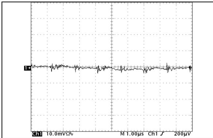
Figure 15: Input reflected ripple current,  $i_s$ , through a  $10\ \mu\text{H}$  source inductor, using a  $47\ \mu\text{F}$  ceramic input capacitor ( $5\ \text{mA}/\text{div}$ ). See Figure 13.
