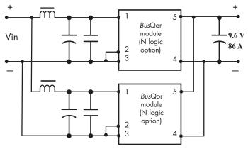
Figure H: BusQor Output Paralleling for increased current output
