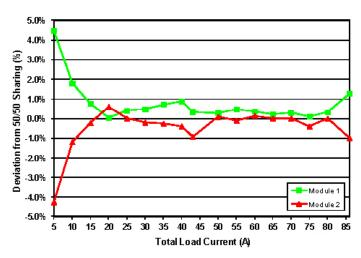
Figure 1: Current share performance of 2 paralleled modules
