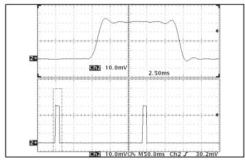
Figure 17: Load current (20 A/div) as a function of time when the converter attempts to turn on into a 1 m $\Omega$  short circuit. Top trace (2.5 ms/div) is an expansion of the on-time portion of the bottom trace.
