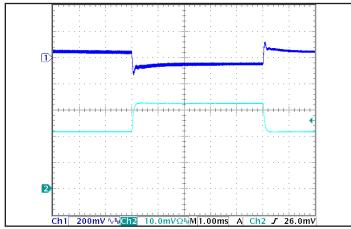
Figure 11: Output voltage response to step-change in load current (50%-75%-50% of lout(max); dI/dt = 0.1 A/ $\mu$ s). Load cap: 15  $\mu$ F, 100 m $\Omega$  ESR tantalum cap and 1  $\mu$ F ceramic cap. Top trace: Vout (200 mV/div), Bottom trace: lout (10 A/div).
