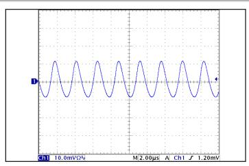
Figure 13: Input Terminal Ripple Current, ic, at full rated output current and nominal input voltage with 10  $\mu$ H source impedance and 47  $\mu$ F electrolytic capacitor (50 mA/div). See Figure 12.
