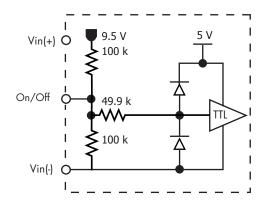
Figure B: Internal ON/OFF pin circuitry
