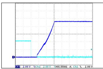
Figure 9: Turn-on transient at half load (resistive load) and 3 mF output capacitance (4.0 ms/div). Input voltage pre-applied. Channel 1: Vout (2 V/div). Channel 2: ON/OFF input (2 V/div).
