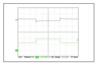
Figure 12: Output voltage response to step-change in load current (50%-75%-50% of lout(max):  $dI/dt = 1 A/\mu s$ ). Load cap: 15  $\mu F$ , 30  $m\Omega$  ESR tantalum cap and 1  $\mu F$  ceramic cap. Ch 1: Vout (500 mV/div), Ch 2: Iout (20 A/div).
