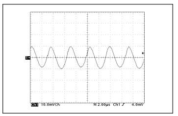
Figure 14: Input Terminal Ripple Current, ic, at full rated output current and nominal input voltage with 10  $\mu$ H source impedance and 47  $\mu$ F electrolytic capacitor (500 mA/div). See Figure 13.
