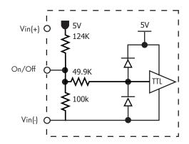
Figure B: Internal ON/OFF pin circuitry
