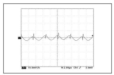
Figure 15: Input reflected ripple current, is, through a  $10~\mu H$  source inductor, using a  $47~\mu F$  electrolytic input capacitor (50 mA/div). See Figure 13.
