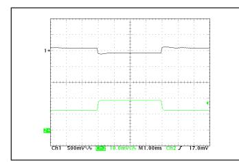
Figure 11: Output voltage response to step-change in load current (50%-75%-50% of lout(max);  $dI/dt = 0.1~A/\mu s$ ). Load cap: 15  $\mu F$  tantalum cap and 1  $\mu F$  ceramic cap. Ch 1: Vout (500 mV/div), Ch 2: lout (20 A/div).
