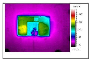
Figure 6: Thermal plot of converter at 37.3 A load current (434 W) with 55  $^{\circ}$ C air flowing at the rate of 200 LFM. Air is flowing across the converter from pin 1 to pin 3 (nominal input voltage).
