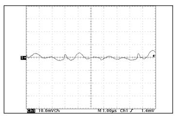
Figure 15: Input reflected ripple current, is, through a  $10\mu H$  source inductor, using a  $47\mu F$  electrolytic input capacitor (20mA/div). See Figure 13.
