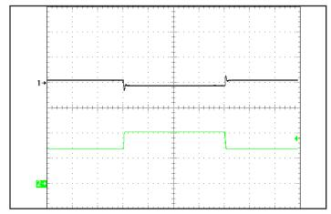
Figure 12: Output voltage response to step-change in load current (50%-75%-50% of lout(max):  $dI/dt = 1A/\mu s$ ). Load cap:  $15\mu F$ , 30 m $\Omega$  ESR tantalum cap and  $1\mu F$  ceramic cap. Ch 1: Vout (1V/div), Ch 2: Iout (25A/div).
