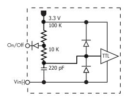
Figure B: Internal ON/OFF pin circuitry
