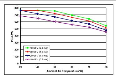
Figure 8: Maximum output power derating curve vs. ambient air temperature (with both baseplate and 0.5" heat sink) at different airflow rates with air flowing from output to input (nominal input voltage).
