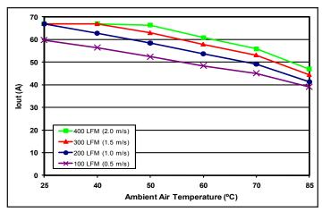
Figure 7: Maximum output current derating curve vs. ambient air temperature (with both baseplate and 0.5" heat sink) at different airflow rates with air flowing from output to input (nominal input voltage).
