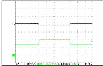
Figure 11: Output voltage response to step-change in load current (50%-75%-50% of lout(max);  $dI/dt = 0.1A/\mu s$ ). Load cap:  $15\mu F$  tantalum cap and  $1\mu F$  ceramic cap. Ch 1: Vout (1V/div), Ch 2: Iout (25A/div).
