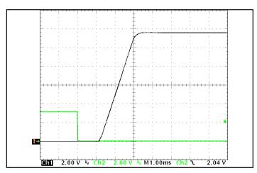
Figure 9: Turn-on transient at half load (resistive load) (1 ms/div). Load cap:  $15\mu F$  tantalum capacitor and 5mF ceramic capacitor bank. Input voltage preapplied. Ch 1: Vout (2V/div). Ch 2: ON/OFF input (2 V/div).
