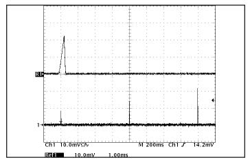
Figure 18: Load current (50A/div) as a function of time when the converter attempts to turn on into a  $Im\Omega$  short circuit. Top trace (Ims/div) is an expansion of the on-time portion of the bottom trace.
