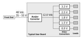
Figure A: Example of Intermediate Bus Architecture using BusQor bus converter and NiQor non-isolated converters
