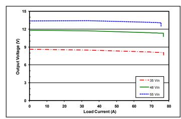
Figure 17: Output voltage vs. load current for different input voltages showing typical current limit curves.
