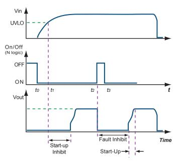
Figure E: Power Up/Down Diagram showing Start-Up Inhibit Period (not to scale)
