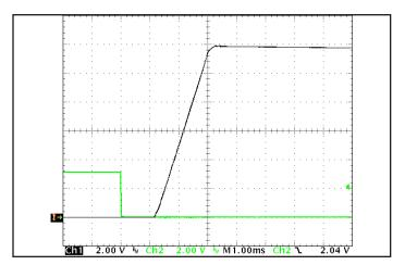
Figure 10: Turn-on transient at zero load (1 ms/div). Load cap:  $15\mu F$  tantalum capacitor and 5mF ceramic capacitor bank. Ch 1: Vout (2V/div), Ch 2: ON/OFF input (2 V/div).
