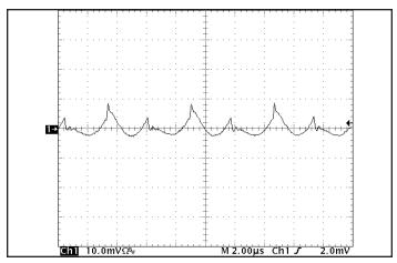
Figure 14: Input Terminal Ripple Current, ic, at full rated output current and nominal input voltage with  $10\mu H$  source impedance and  $47\mu F$  electrolytic capacitor (500 mA/div). See Figure 13.
