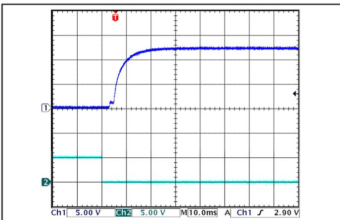
Figure 11: Turn-on transient at full load (resistive load) (10 ms/div). Input voltage pre-applied. Top Trace: V<sub>out</sub> (5V/div). Bottom Trace: ON/OFF input (5V/div)
