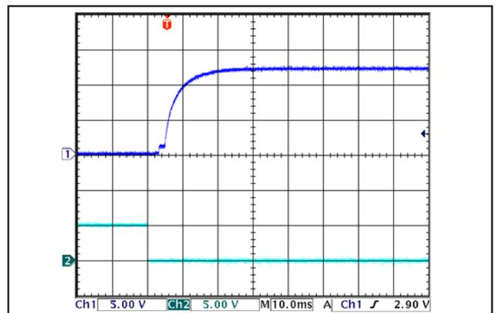
Figure 12: Turn-on transient at zero load (10 ms/div). Top Trace: V<sub>out</sub> (5V/div). Bottom Trace: ON/OFF input (5V/div).
