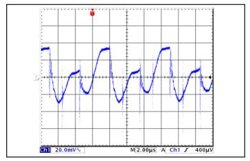
Figure 18: Output voltage ripple at nominal input voltage and rated load current (20mV/div). Load capacitance: 2x22 µF ceramic capacitor. Bandwidth: 500 MHz. (Fig 15)
