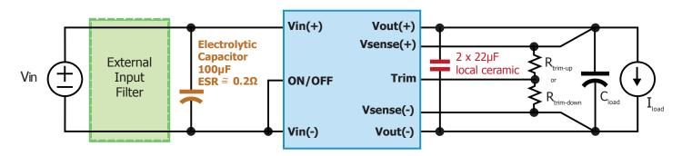
Figure C: Typical Application Circuit (negative logic unit, permanently enabled).
