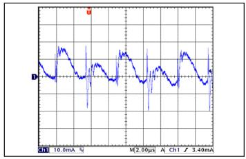
Figure 17: Input reflected ripple current, is, through a 4.7 µH source inductor at nominal input voltage and rated load current (10mA/div). (Fig 15)
