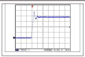
Figure 20: Load current (10A/div) as a function of time when the converter attempts to turn on into a  $Im\Omega$  short circuit.
