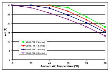
Figure 7: Max output power derating curves vs. ambient air temperature for airflow rates of 100 LFM through 400 LFM with air flowing across the converter from input to output (nominal input voltage).
