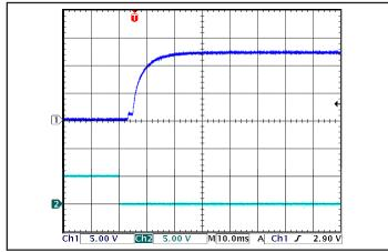
Figure 11: Turn-on transient at full load (resistive load) (10 ms/div). Input voltage pre-applied. Top Trace: Vout (5V/div). Bottom Trace: ON/OFF input (5V/div) div)
