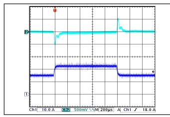
Figure 13: Output voltage response to step-change in load current (50%-75%-50% of lout(max);  $dI/dt = 0.1A/\mu$  s). Load cap: 47  $\mu$ F ceramic cap. Top trace: Vout (500mV/div), Bottom trace: lout (10A/div).
