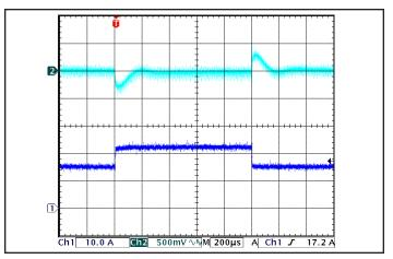
Figure 14:Output voltage response to step-change in load current (50%-75%-50% of lout(max):  $dI/dt = 5A/\mu$  s). Load cap: 470  $\mu$ F, 15  $m\Omega$  ESR tantalum cap and 47  $\mu$ F ceramic cap. Top trace: Vout (500mV/div), Bottom trace: lout (10A/div)
