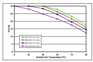
Figure 9: Max output power derating curves vs. ambient air temperature for airflow rates of 100 LFM through 400 LFM with air flowing from pin 1 to pin 4 (nominal input voltage).
