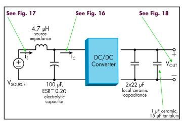
Figure 15:Test set-up diagram showing measurement points for Input Terminal Ripple Current (Fig 16), Input Reflected Ripple Current (Fig 17) and Output Voltage Ripple (Fig 18).
