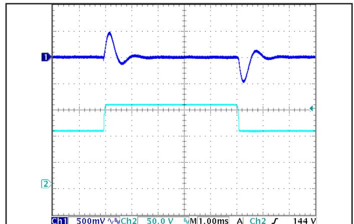
Figure 6: Output voltage response to step-change in input voltage (nominal to maximum input voltage), at Full Load current. Load cap: 1 uF ceramic cap. Ch 1: V<sub>out</sub>, Ch 2: V<sub>in</sub>.
