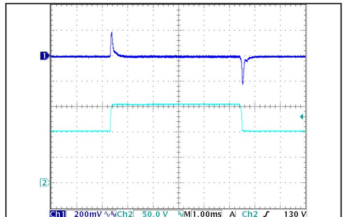
Figure 6: Output voltage response to step-change in input voltage (nominal to maximum input voltage), at Full Load current. Load cap: 15 μF tantalum capacitor and 1 μF ceramic cap. Ch 1: V<sub>out</sub>, Ch 2: V<sub>in</sub>.
