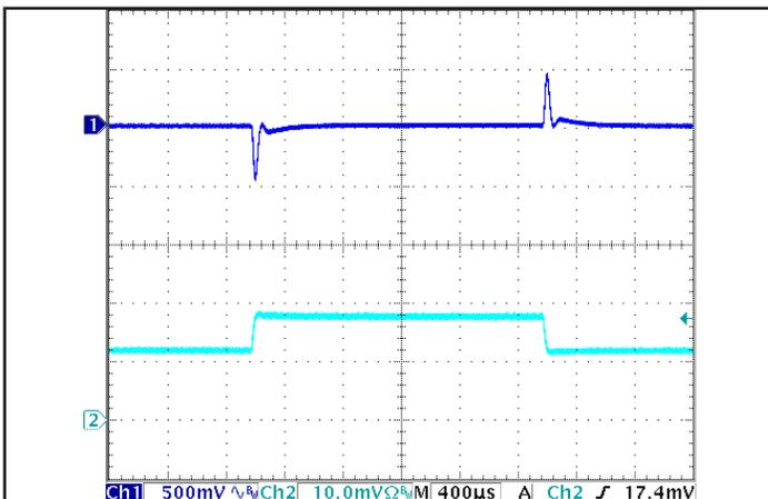
Figure 5: Output voltage response to step-change in load current (50% -75% -50% of I<sub>out</sub>(max); dI/dt = 0.1 A/μs). Load cap: 15 μF tantalum cap and 1 μF ceramic cap. Ch 1: V<sub>out</sub>, Ch 2: I<sub>out</sub>. (5 A/div.)
