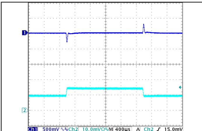
Figure 5: Output voltage response to step-change in load current (50% -75% -50% of I<sub>out</sub>(max); dI/dt = 0.1 A/μs). Load cap: 15 μF tantalum cap and 1 μF ceramic cap. Ch 1: V<sub>out</sub>, Ch 2: I<sub>out</sub>. (10 A/div.)
