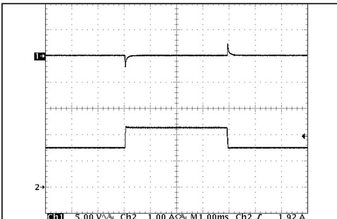
Figure 5: Output voltage response to step-change in load current (50 % -75 % -50 % of I<sub>out</sub>(max); dI/dt = 0.1 A/μs). Load cap: 15 μF tantalum cap and 1 μF ceramic cap. Ch 1: V<sub>out</sub>, Ch 2: I<sub>out</sub>.
